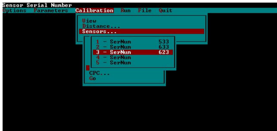
Figure 2.2.6.10 Sensor serial number menu (serial numbers shown will be different from values shown on the figure).
