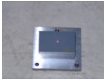
Figure 2.5.4.8. Block on top of base plate with calibration plate on top of block.
