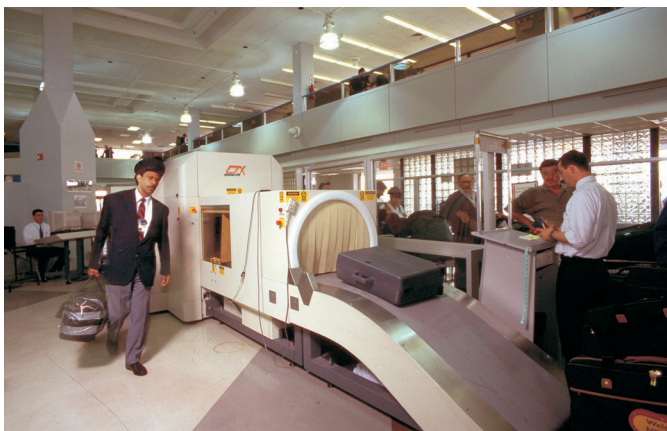
Explosive detection systems are just one technology to ensure that passenger bags are properly screened.
