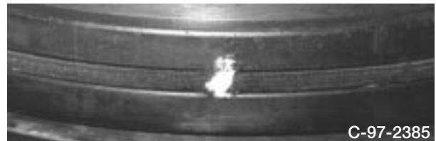
Figure 11.—Photo of 1/16 in. diameter hybrid seal after hot scrubbing, 0.014 in. linear seal compression (minor lap joint damage only).
