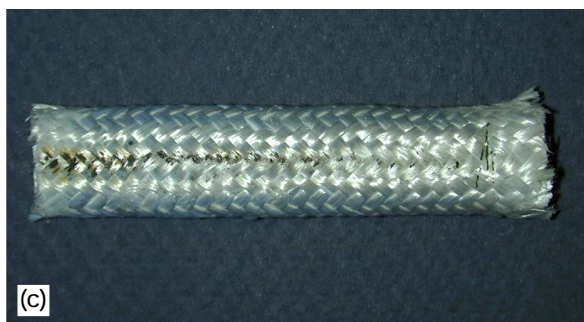
Figure 7.—Photos of 6 pcf X-38 seals before and after 1900 °F temperature exposure. (a) Side-by-side photo of seals before (left) and after (right) temperature exposure. (b) Photo of seal before exposure showing condition of ceramic outer layer. (c) Photo of seal after exposure showing condition of ceramic outer layer.
