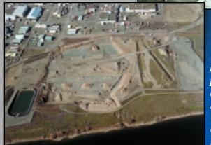
East of DR Reactor, 66-inch effluent water lines that lead to retention basins and on to the river are being removed. More than half of the reactor's footprint has been removed as part of the Reactor Interim Safe Storage Project.
