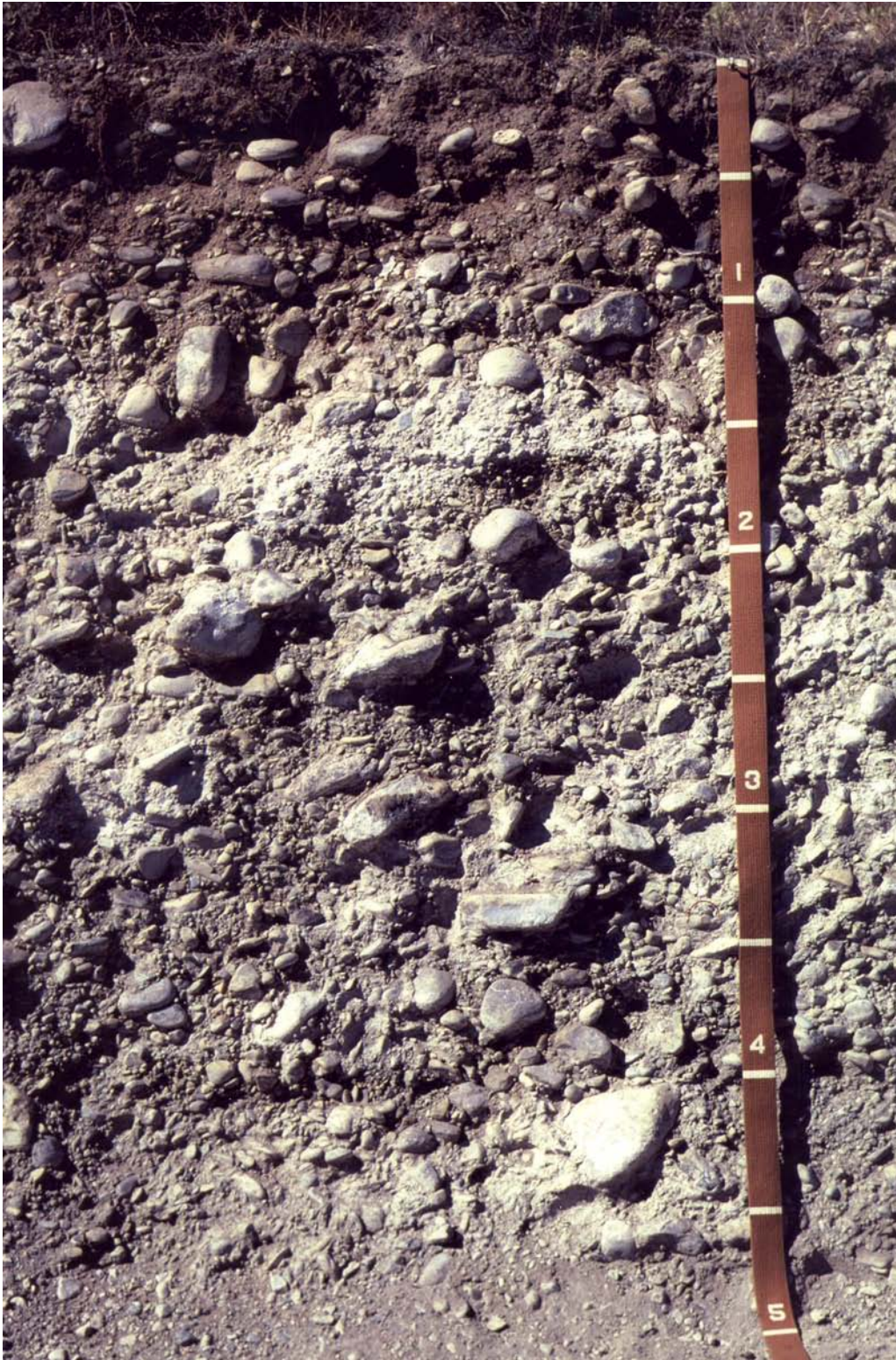
Figure 13.—Typical profile of Whiteknob gravelly loam, 2 to 8 percent slopes. This soil formed in alluvium derived from quartzite. Lime and silica coatings on underside of rock fragments between depths of 7 and 60 inches. The numerals on the tape are in feet.
