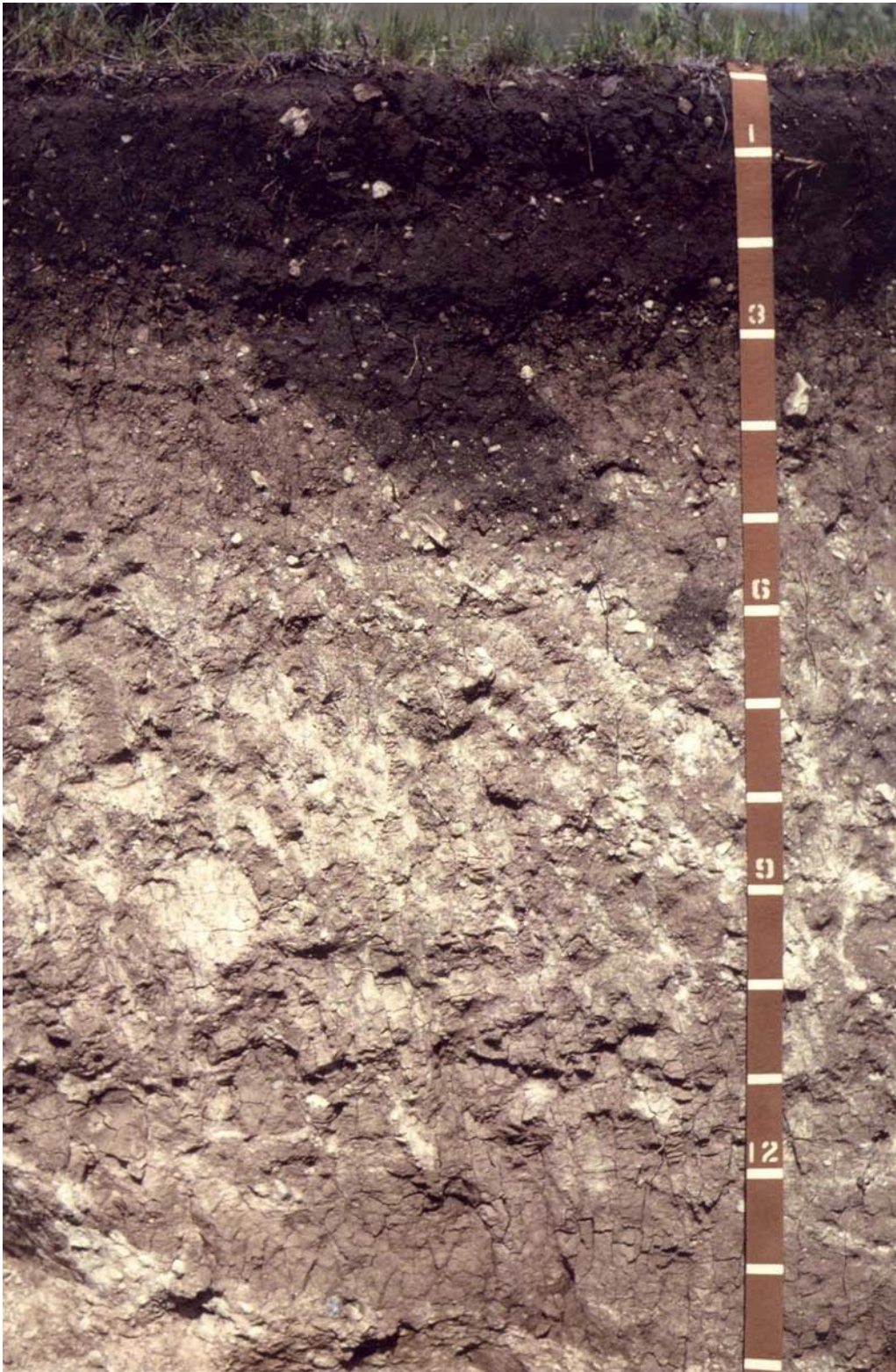
Figure 8.—Typical profile of Heathcoat gravelly silt loam, 4 to 20 percent slopes. This soil formed in uplifted lacustrine and alluvial material over glacial till. The dark-colored surface layer and subsoil extend to a depth of 28 centimeters (11 inches). The numerals on the tape are in decimeters.
