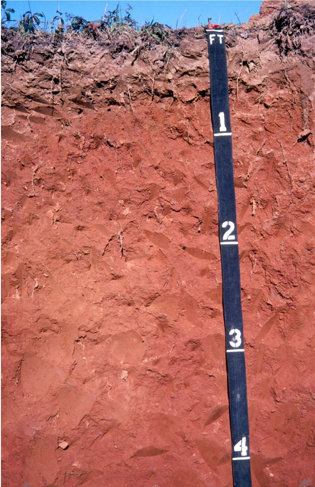
Figure 15.—A profile of a Lucedale soil. Lucedale soils formed in thick deposits of loamy sediments. They are very deep, are loamy, and are dark red throughout the subsoil. They are on summits of high terraces.
