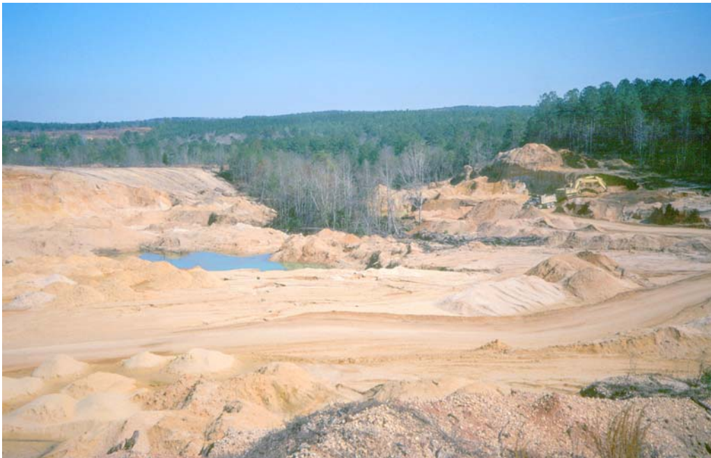
Figure 8.—A large sand and gravel pit, map unit Pg, near Rabbit Creek, northeast of Jackson. This area was formerly Flomaton-Smithdale-Wadley complex, 10 to 25 percent slopes. The layers of sand and gravel are several feet thick and the deposits are presumed to be of Pleistocene or Pliocene age.
