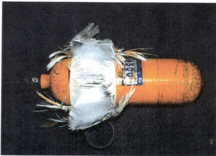
Figure 6. Failure Region of Accident SCBA Cylinder
