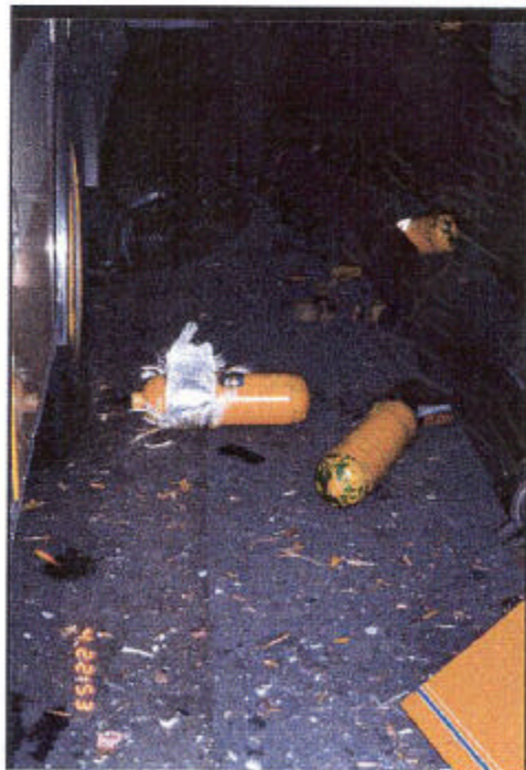
Figure 2. View of Failed Cylinder after Accident
