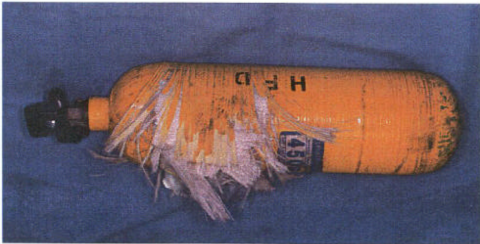
Figure 8. Initial Failure Region of Accident SCBA Cylinder
