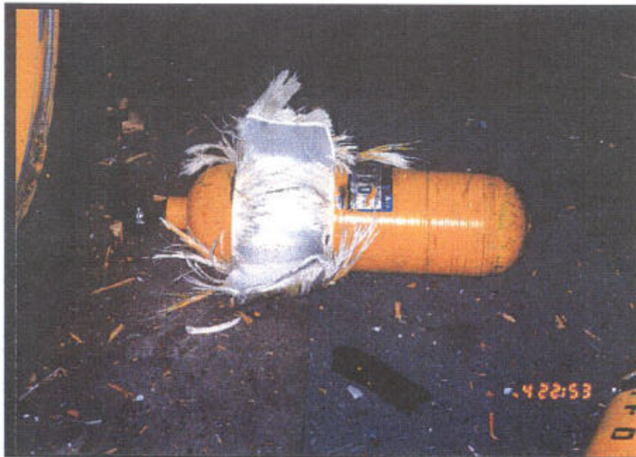
Figure 3. Close-up View of Failed Cylinder after Accident
