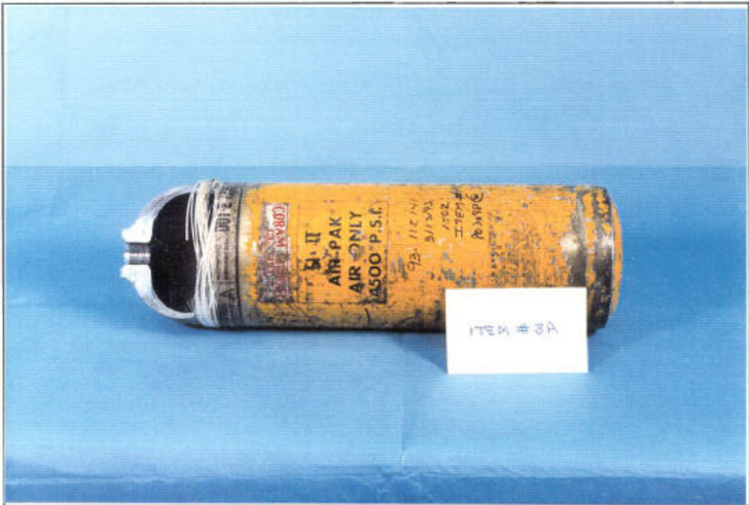
FIGURE 6 SCOTT AIR PAK CYLINDER THAT RUPTURED AT NECK -- ITEM 3A
