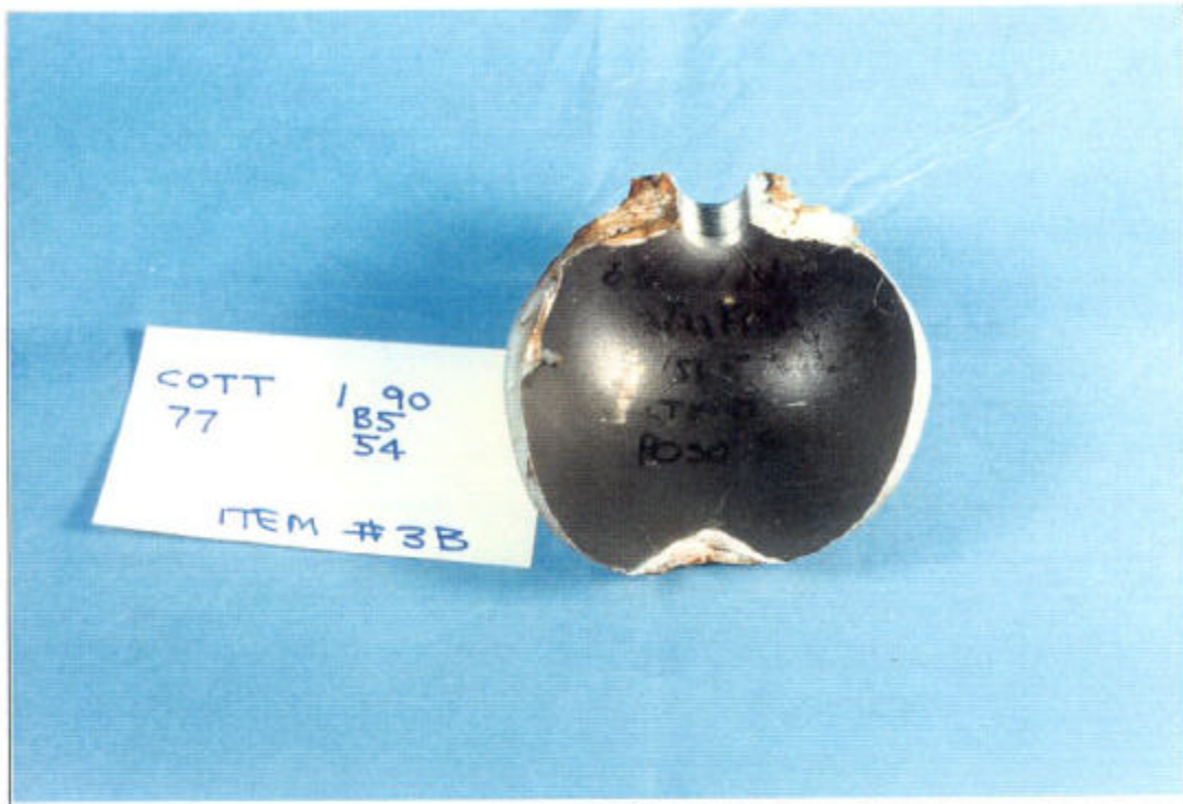
FIGURE 7 FRAGMENT OF SCOTT AIR PAK CYLINDER THAT RUPTURED -- ITEM 3A
