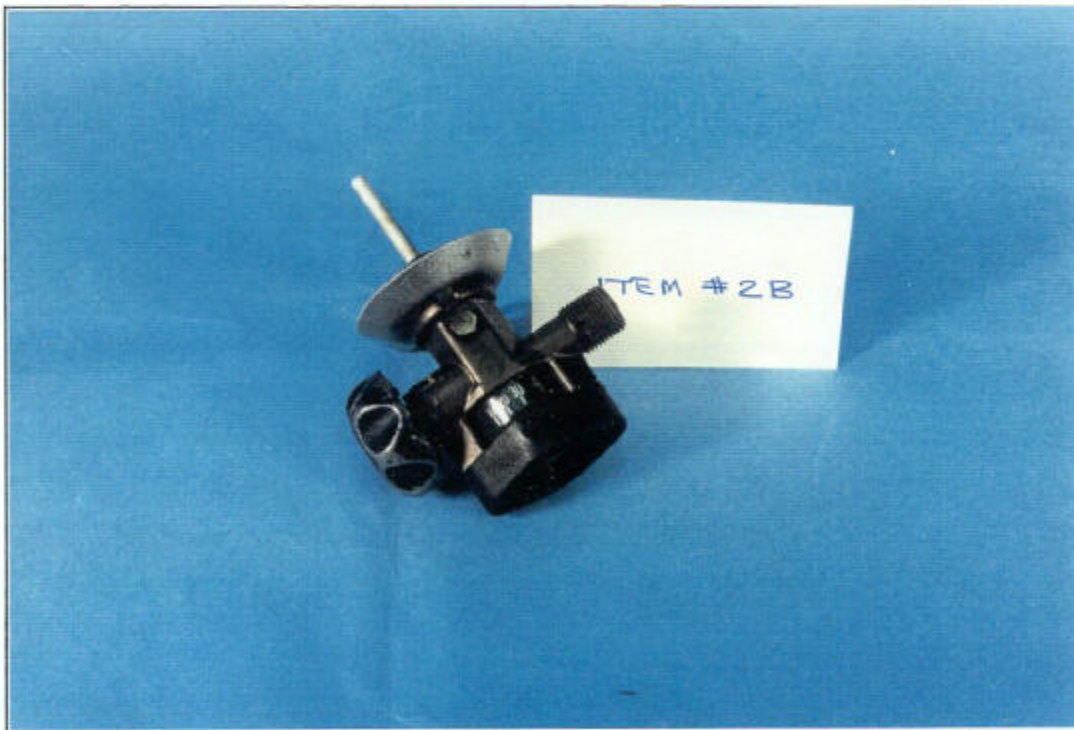
FIGURE 4 VALVE SYSTEM REMOVED FROM ITEM 2A
