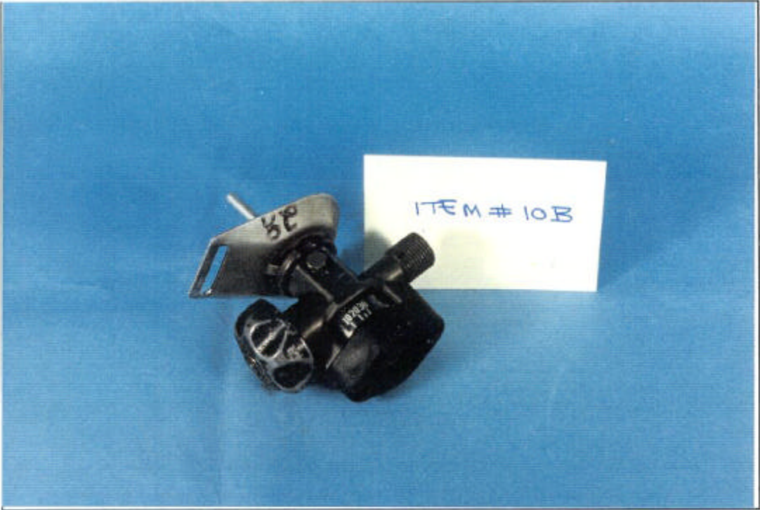
FIGURE 5 VALVE SYSTEM REMOVED FROM ITEM 10A
