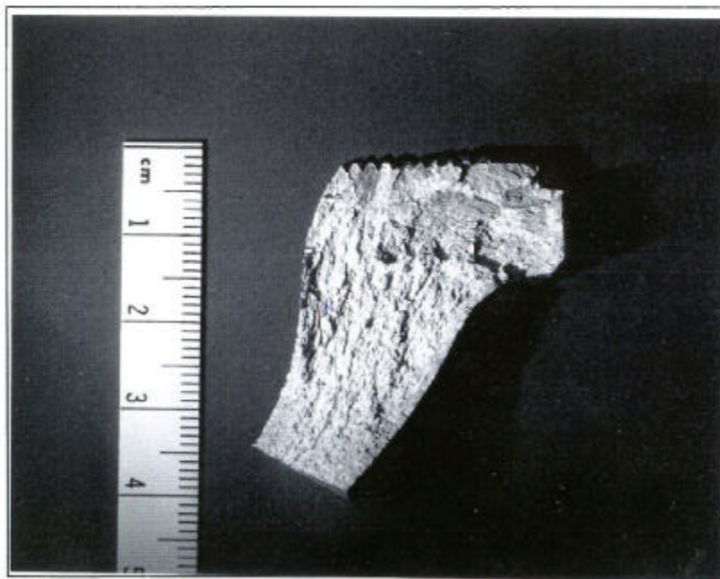
FIGURE 22 SPECIMEN FROM THE SHOULDER OF THE RUPTURED CYLINDER USED FOR MICROSCOPIC EXAMINATION
