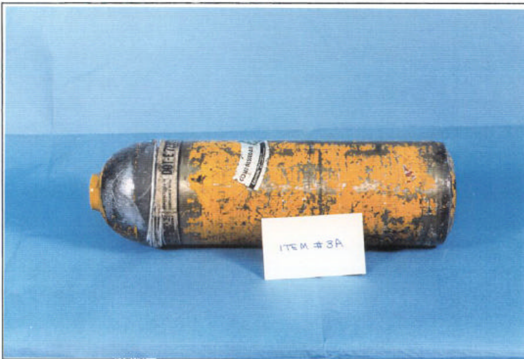
FIGURE 14 MARKING IDENTIFYING THE RUPTURED CYLINDER AS A TYPE DOT-E-7235
