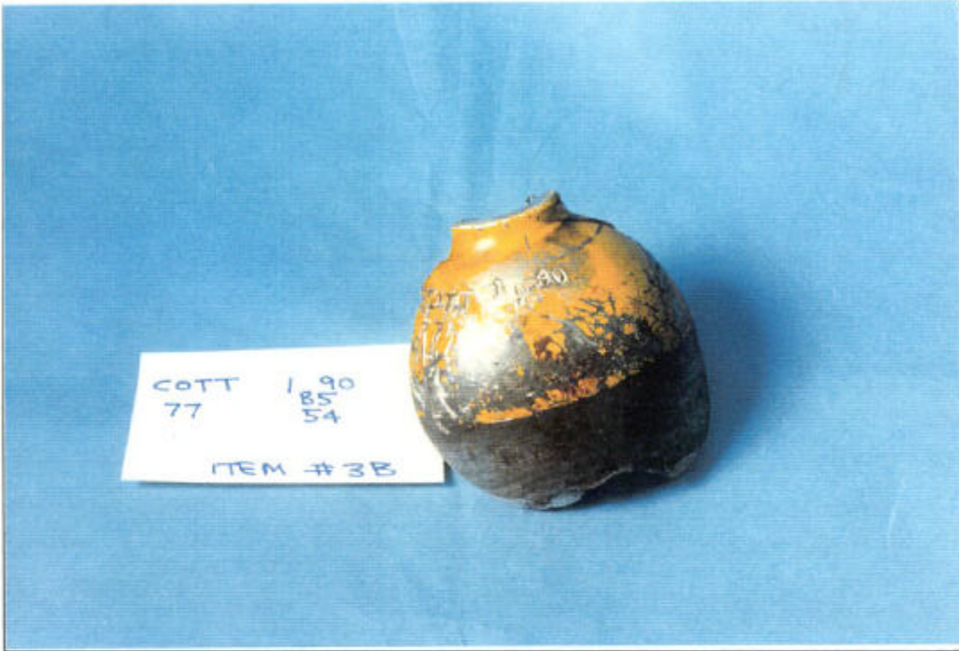
FIGURE 17 MARKINGS ON THE HEAD OF THE CYLINDER THAT RUPTURED SHOWING THE YEAR OF MANUFACTURE -- ITEM 3B
