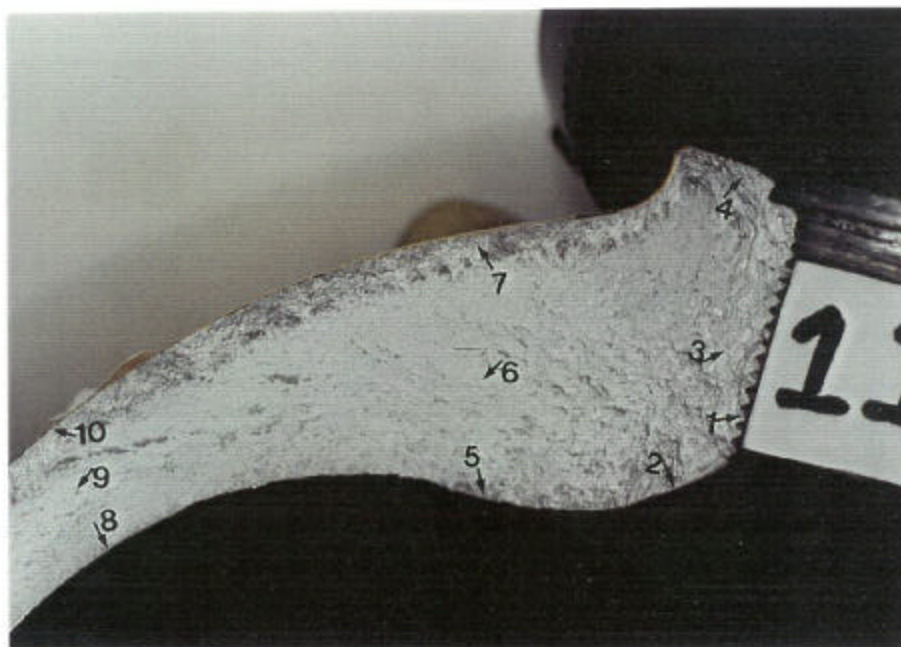
Figure 20. A macro view of the fracture surface #1 which was examined to characterize the fracture features. Areas indicated by arrowed numbers were examined at higher magnifications under the SEM.
