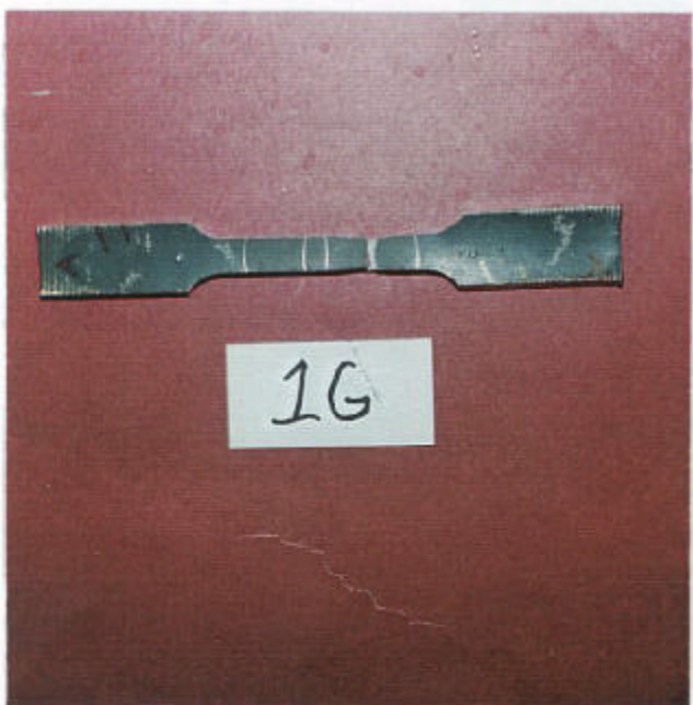
Figure 7. Tested longitudinal tensile coupon (1G) having a 48.0 ksi 0.2% yield strength, 51.5 ksi ultimate tensile strength, and 19.3% elongation in 2.0 in. and remaining upper fracture edge section of (1H) of the cylindrical wall shown in Figure 2.
