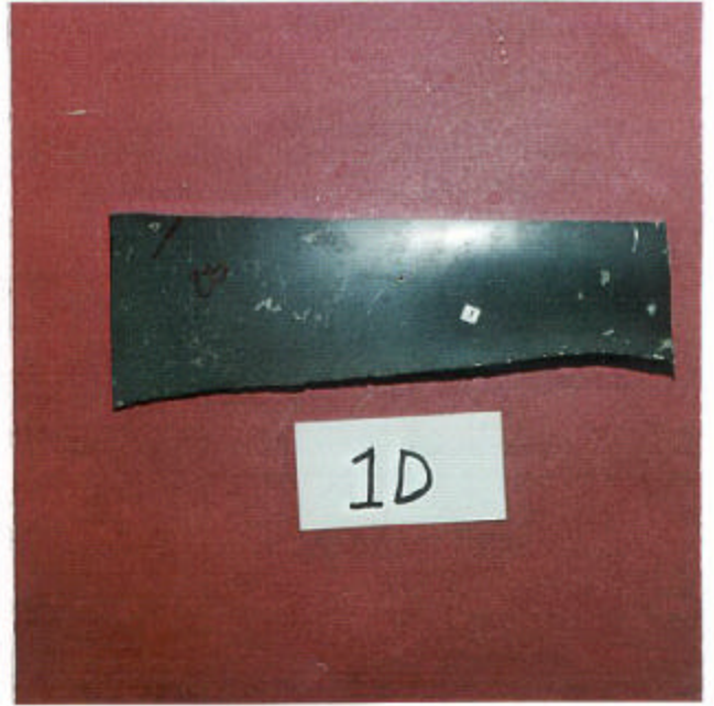
Figure 5. Tested longitudinal tensile coupon (1C) from lower center section having a 47.7 ksi 0.2% yield strength, 51.7 ksi ultimate tensile strength and 15.5% elongation in 2 in. and remaining lower right fracture edge section (1D) shown in Figure 2.
