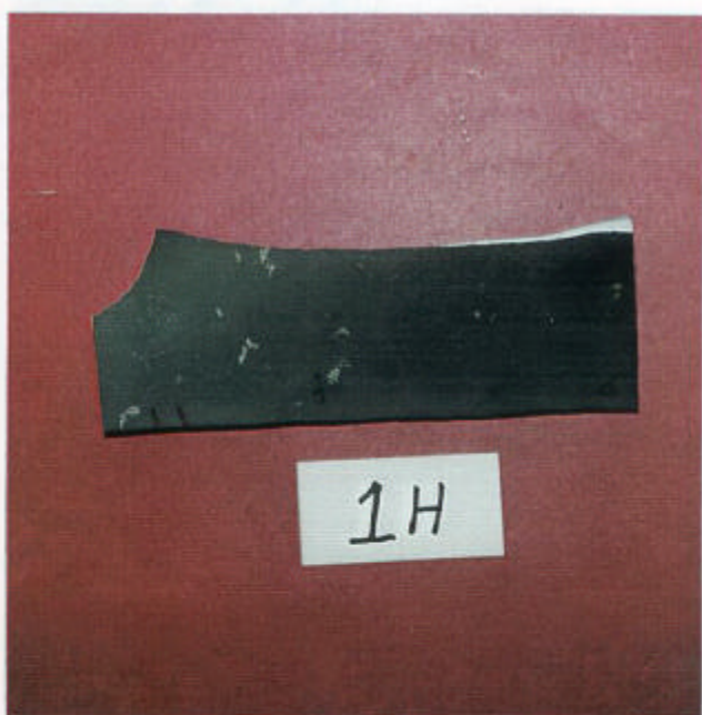
Figure 7. Tested longitudinal tensile coupon (1G) having a 48.0 ksi 0.2% yield strength, 51.5 ksi ultimate tensile strength, and 19.3% elongation in 2.0 in. and remaining upper fracture edge section of (1H) of the cylindrical wall shown in Figure 2.
