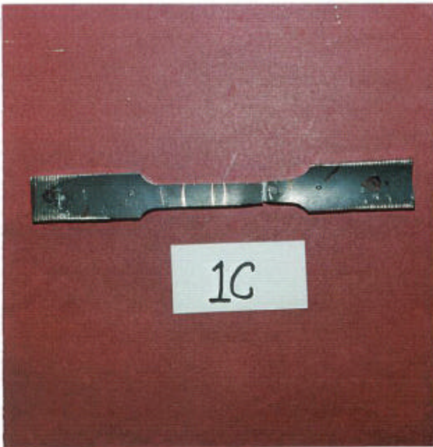
Figure 5. Tested longitudinal tensile coupon (1C) from lower center section having a 47.7 ksi 0.2% yield strength, 51.7 ksi ultimate tensile strength and 15.5% elongation in 2 in. and remaining lower right fracture edge section (1D) shown in Figure 2.
