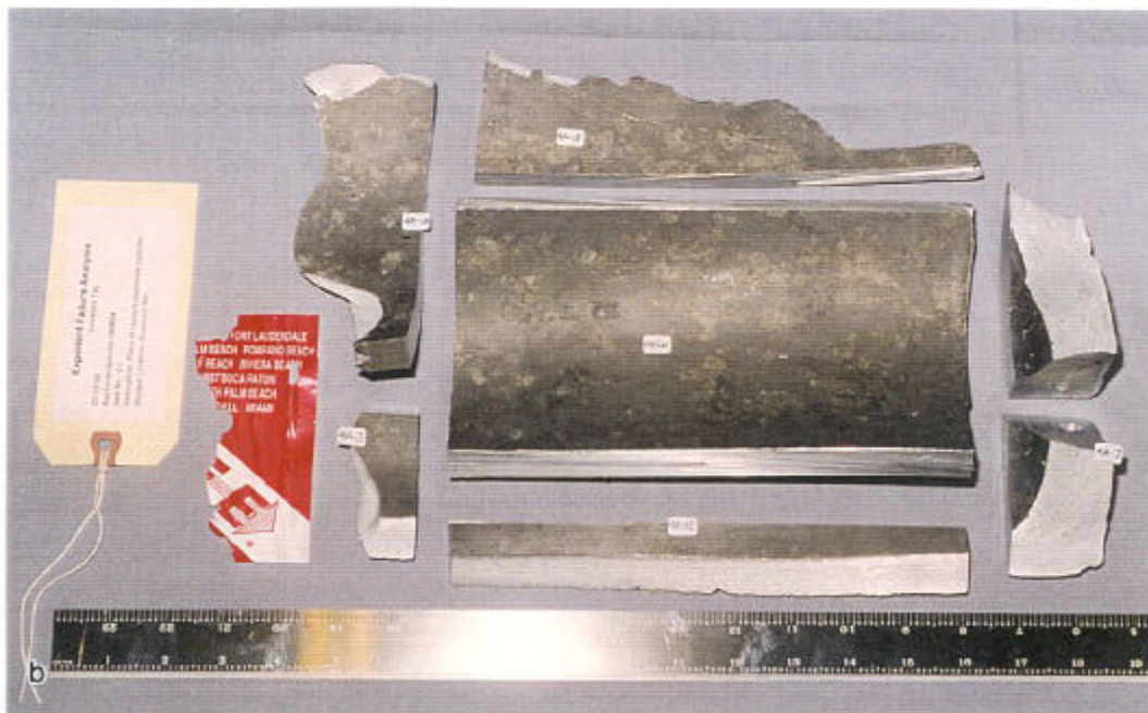
Figure 5. Sectioning of fragment 4A. (a) Initial cuts showing the locations of drilling for chemical composition determination. Photo ID: DC18129-R3E16. (b) Sectioning showing separated fracture surfaces and the portion used for tensile testing. Photo ID: DC18129-R5E3.
