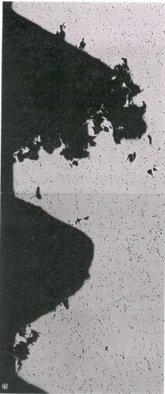
Figure 8. Close-up of thread area shown in Figure 7. (a) 50X. Photo ID: DC18129-PAL-5,6-7/28/98. (b) 50X. HF-H 2 SO 4 -H 2 O etch. Photo ID: DC18129-PAL-9,10-7/28/98. Note the corrosion pitting damage to the thread area.
