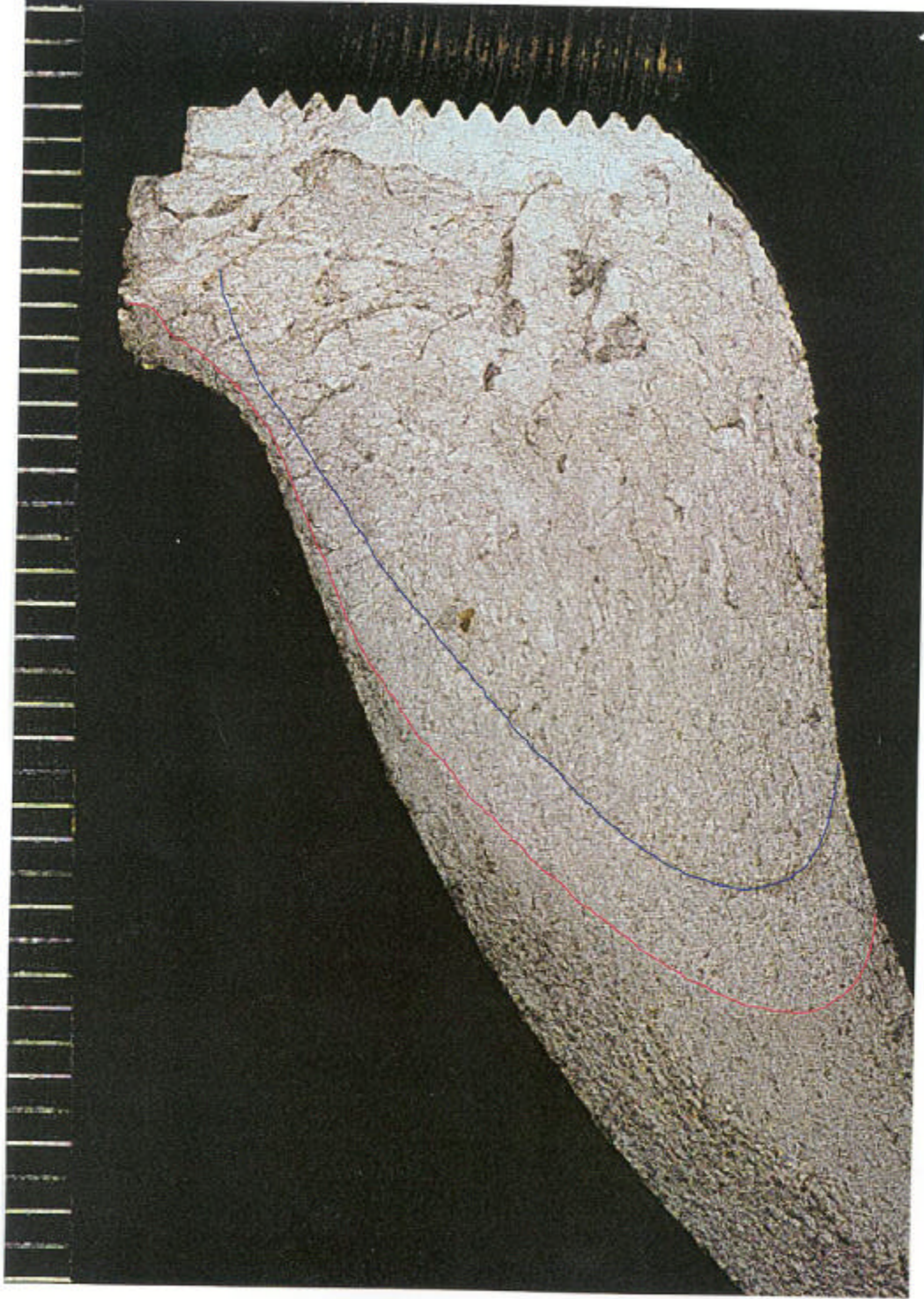
Figure 18: Fracture surface 1A-1, showing crack fronts at different time points (beach marks).
