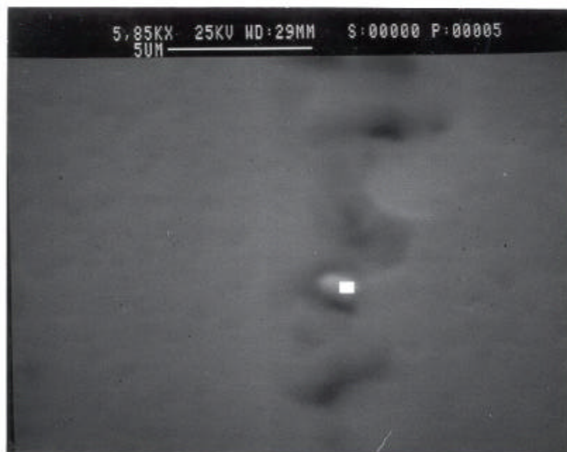
Figure 41A: SEM micrograph showing the spot on a precipitate particle which was analyzed using EDS, X5850.
