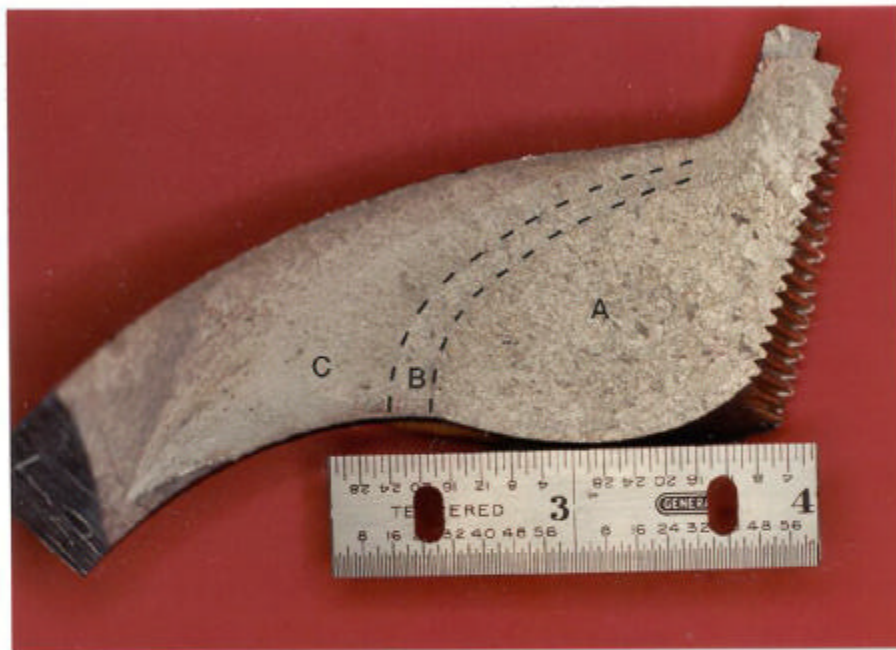
Figure 20: An enlarged view of section 1 (figure 18B) shows three distinct regions on the fracture surface marked A, B and C.
