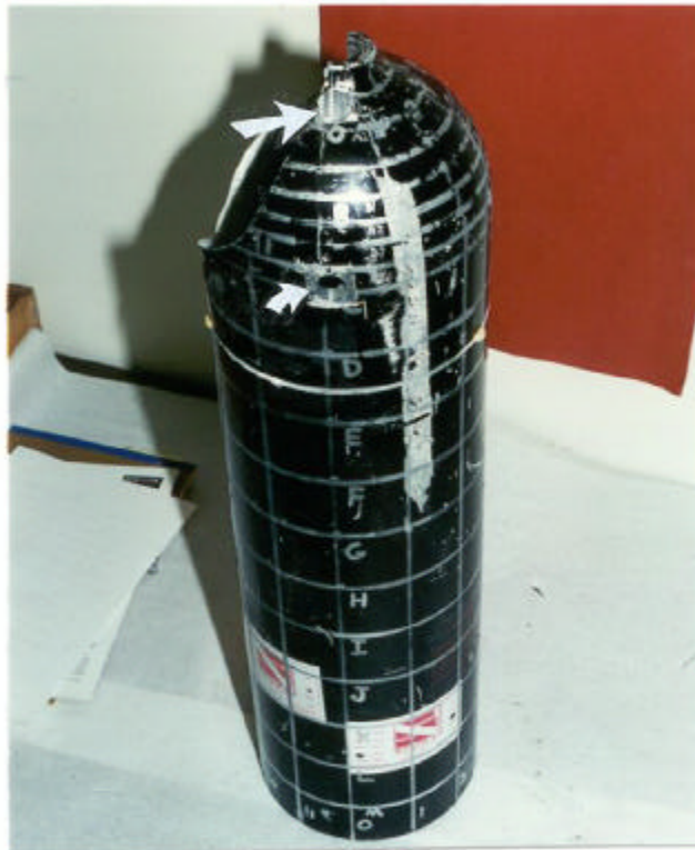
Figure 18A: Locations of chemical samples from near OC grid point (small arrow), and from near OA2 grid point (large arrow).
