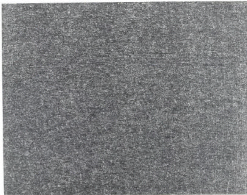
Section 32: Enlarged view of the area marked 1 in figure 31 shows a very fine grain size, X10.
