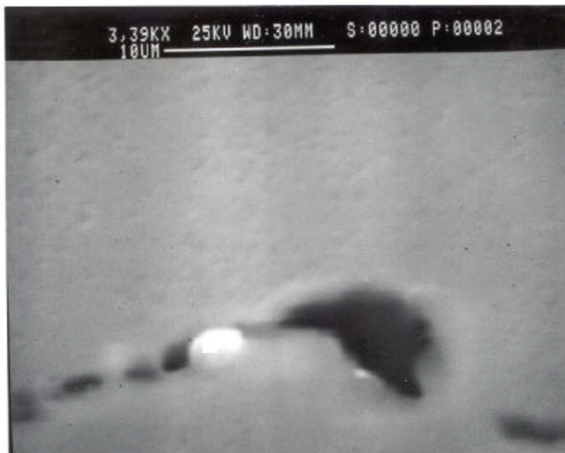
Figure 40A: SEM micrograph exhibits the spot on a precipitate particle which was analyzed using EDS, X3390.
