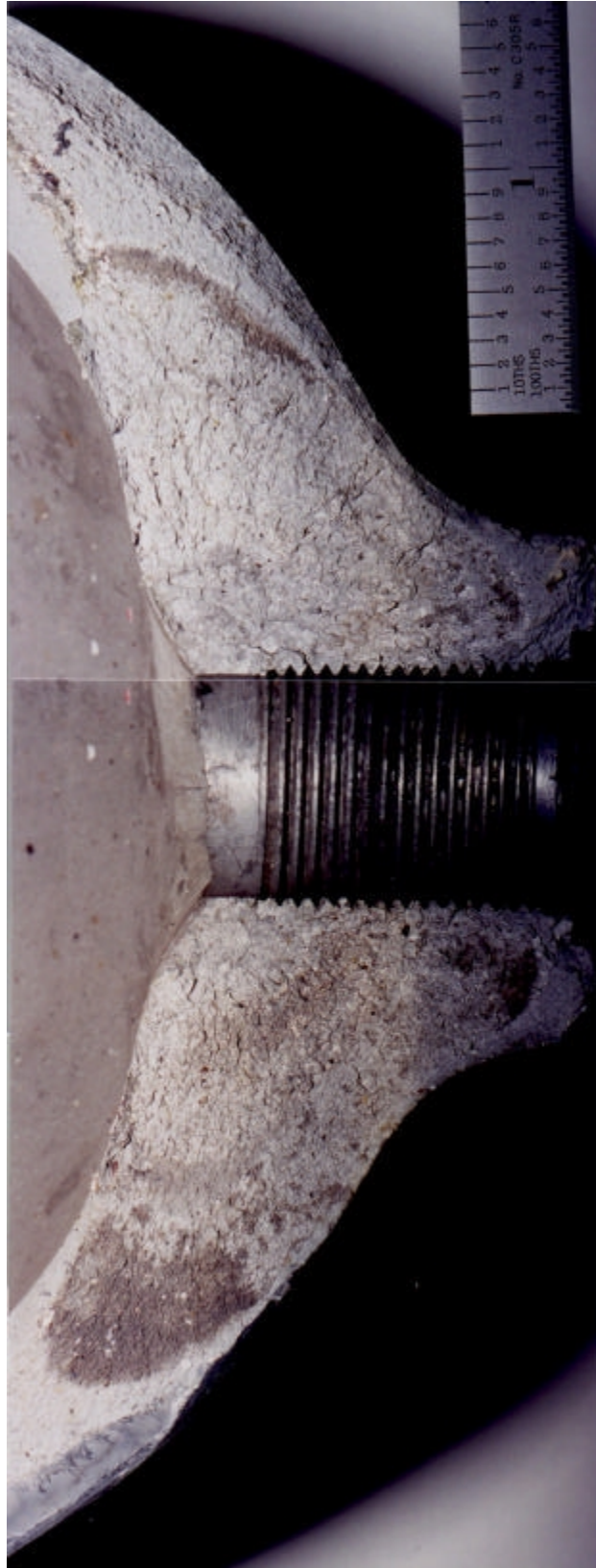
Figure 3. Photomontage of the fracture surface in the neck region. DC18344-R6E14,15.
