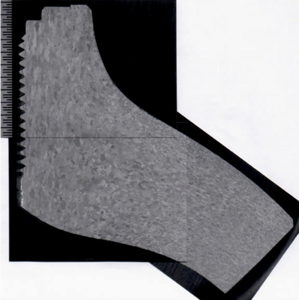
Figure 7. Microstructure of the neck region. Photo ID: DC18344-PAL-4,5,6-8/30/00.
