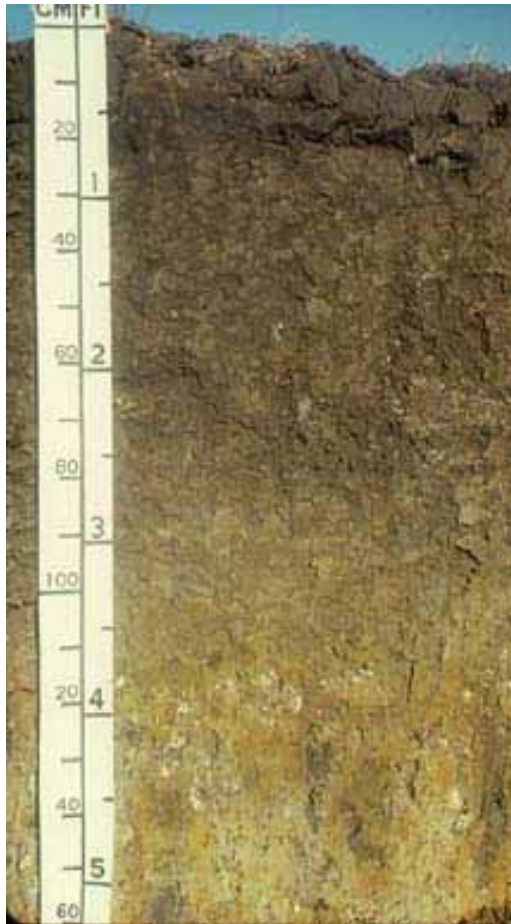
Figure 32.—Profile of Labelle silt loam, 0 to 1 percent slopes. The dark colored loamy surface contacts the clayey subsoil at a depth of 1.25 feet. Concretions of calcium carbonate occur at a depth of 4 feet.
