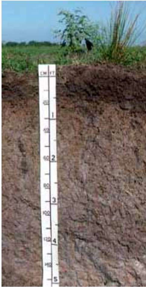
Figure 30.—Profile of Beaumont clay, 0 to 1 percent slopes. A relatively thin dark colored surface layer about 6 inches thick lies on top of the gray clayey subsoil.
