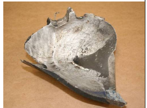
Figure 2: DOT 3AL Cylinder Rupture
