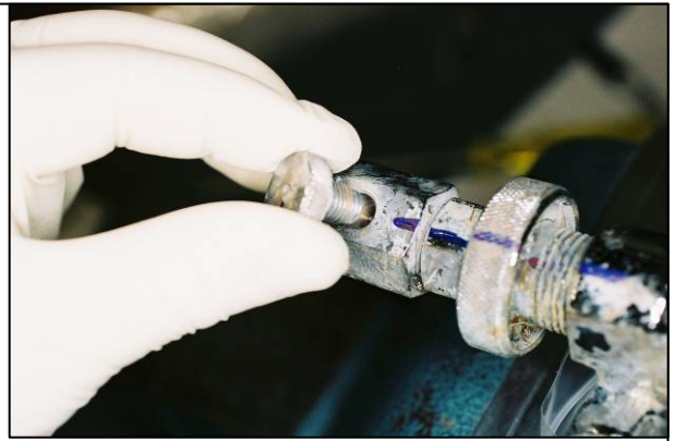
Figure 17 – Cylinder Valve Adaptor Fitting Bleed Valve Disassembly
