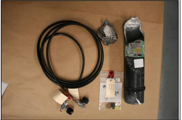
Figure 2: DOT 3AL Cylinder Rupture
