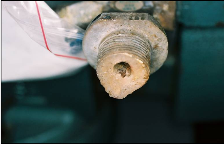
Figure 20 - Particulate Residue Removed From Cylinder Valve Inlet Bore
