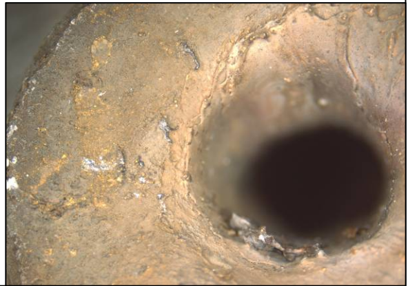
Figure 20 - Particulate Residue Removed From Cylinder Valve Inlet Bore
