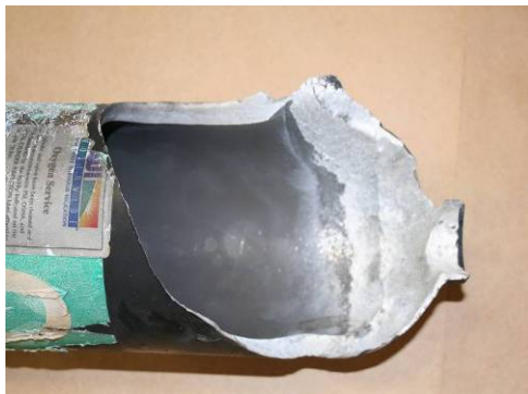
Figure 2: DOT 3AL Cylinder Rupture
