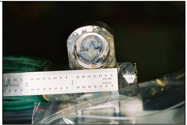
Figure 21 – Cylinder Valve Outlet Condition (Debris Collection)
