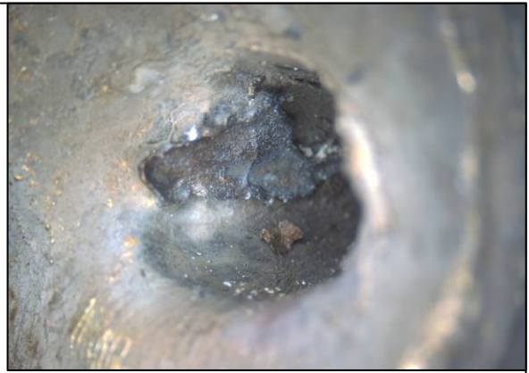
Figure 19 – Cylinder Valve Inlet Debris
