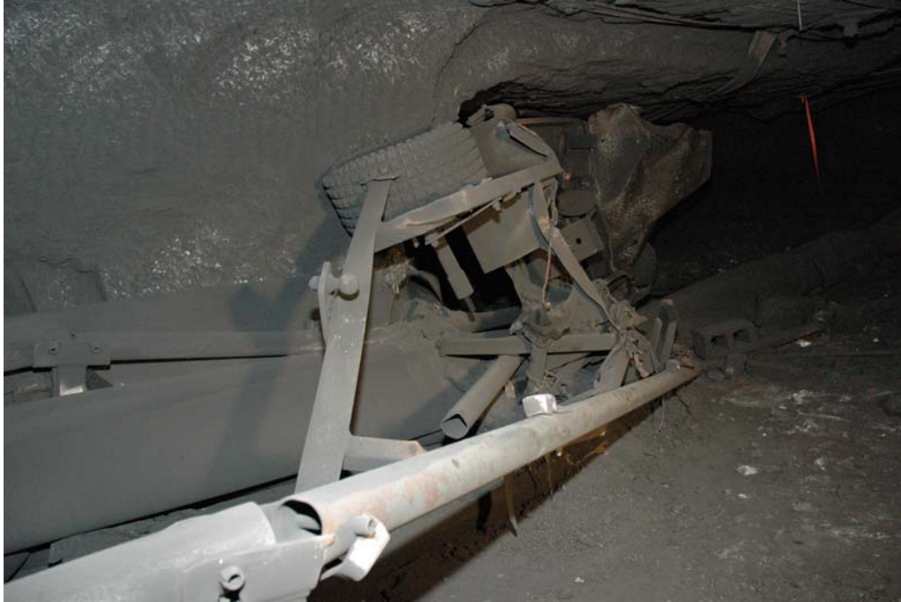
Figure 6 - Damaged Personnel Carrier on top of Conveyor Belt Debris
