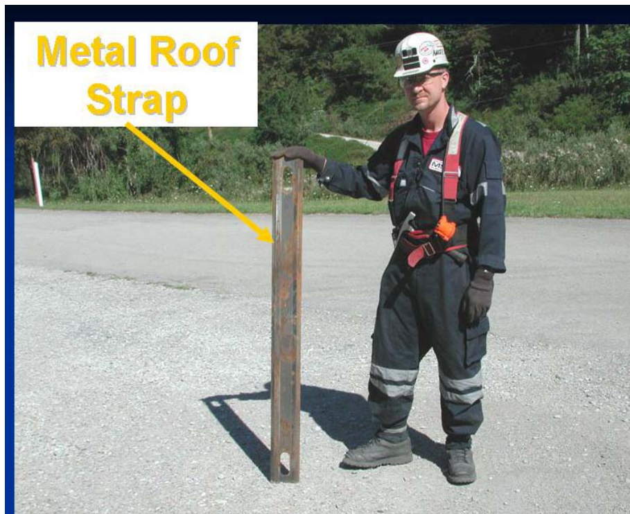
FIGURE 1. MSHA EMPLOYEE HOLDING METAL ROOF STRAP
