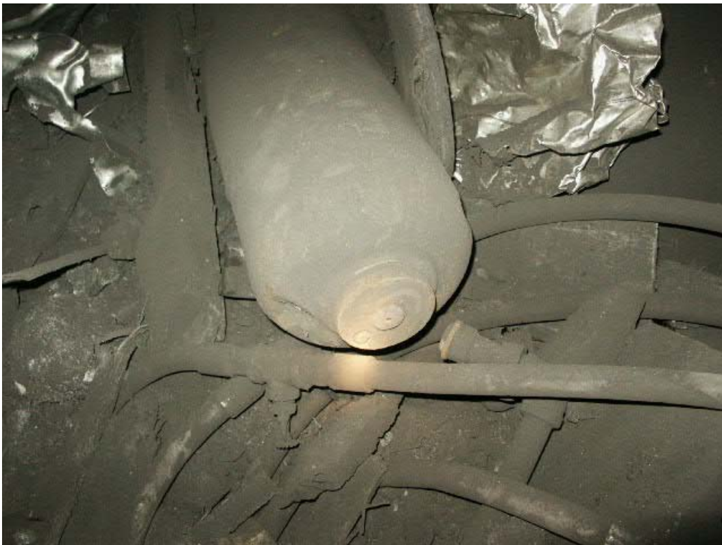
Photograph 10 - Acetylene cylinder found in the No. 5 Entry
