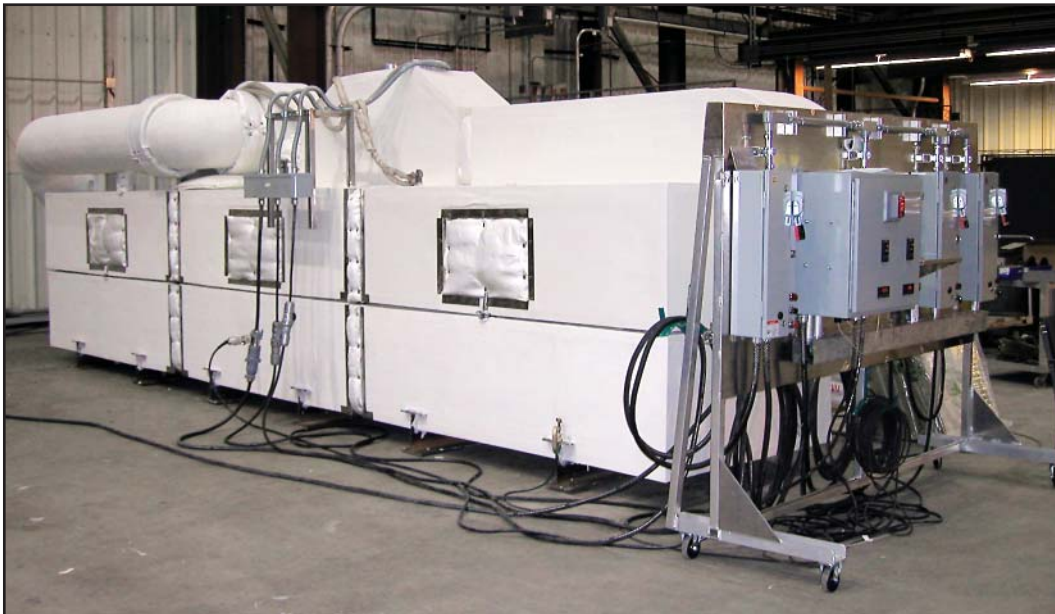
Figure 4. The new oven designed and built at PPPL for the press molding and curing of NSTX's redesigned TF inner bundle.
