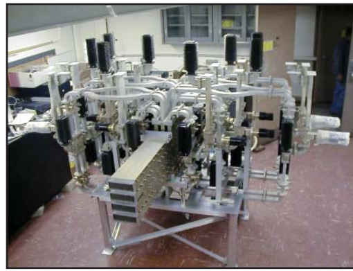
Figure 16. The lower-hybrid launcher's rear waveguide following assembly at PPPL. This component includes interfaces to the microwave power sources, microwave power splitter, directional couplers to measure forward and reflected microwave power, and phase shifters to provide the proper wave front to the plasma.
