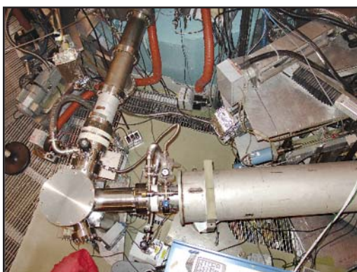
Figure 17. The NSTX X-ray crystal spectrometer installed on the Alcator C-Mod at the Massachusetts Institute of Technology. The Alcator C-Mod tokamak is at the top middle of the picture, the X-ray crystal spectrometer is under the circular plate at the lower left, and the position-sensitive X-ray detectors and electronic equipment are outside the picture to the right.
