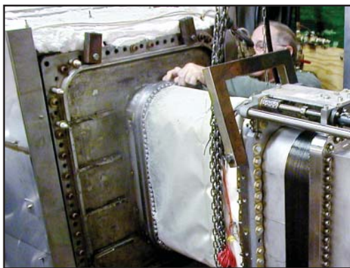
Figure 15. The lower-hybrid launcher's forward waveguide on the PPPL vacuum test stand. This component includes a radial drive system to vary the coupler/plasma separation and optimize microwave power deposition in the plasma.
