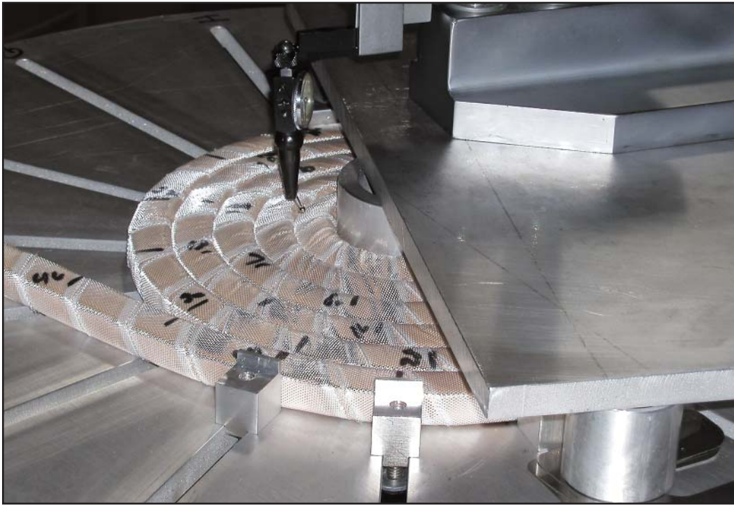
Figure 8. Conductor keystone test done on the NCSX modular coils.
