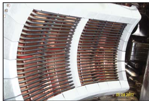
Figure 5. The PPPL-designed four-strap ion-cyclotron radio-frequency antenna, as installed and modified in conjunction with the Plasma Science and Fusion Center at the Massachusetts Institute of Technology.
