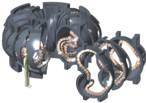
Figure 7. National Compact Stellarator Experiment modular coil assembly.
