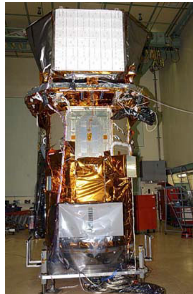
In Building 7's cleanroom, the BAT instrument is integrated on top of the Swift hardware.
