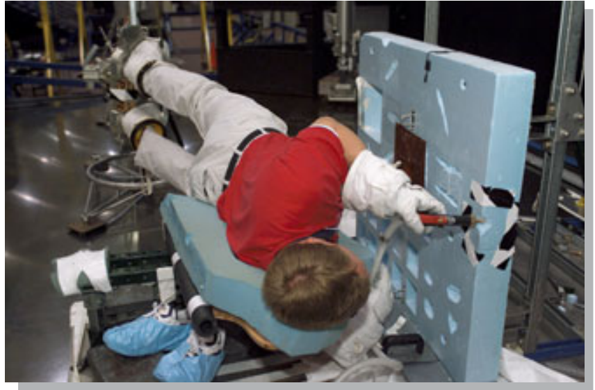
Astronaut Scott E. Parazynski uses an air-bearing floor to approximate some of the conditions of an in-space extravehicular activity (EVA) that might be called upon to repair damaged thermal tiles on a space shuttle.
