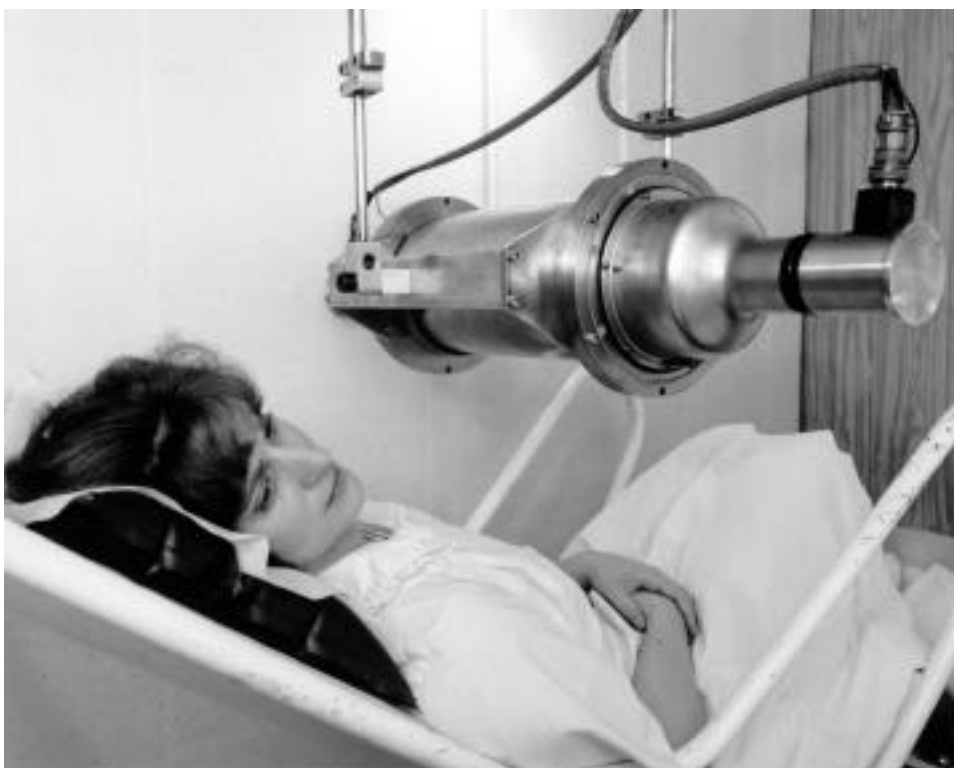
FIGURE 8 Inside the whole-body counter in Argonne's Center for Human Radiobiology, a patient is ready for a measurement of gamma rays emitted from her body. The patient wears clean clothing supplied by the Center and reclines on a metal chair beneath the cylindrical NaI(Tl) crystal that serves as the detector.
