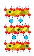
Ultimately, the anion exchange ability and anion selectivity of LDHs are dictated by the number and arrangements of the different cations in the sheets of the structure. Therefore, to understand how to tailor LDHs for a particular application, it is first necessary to understand the cation distribution. Conventional diffraction and spectroscopy methods to characterize LDH structures have proved inadequate, so the
