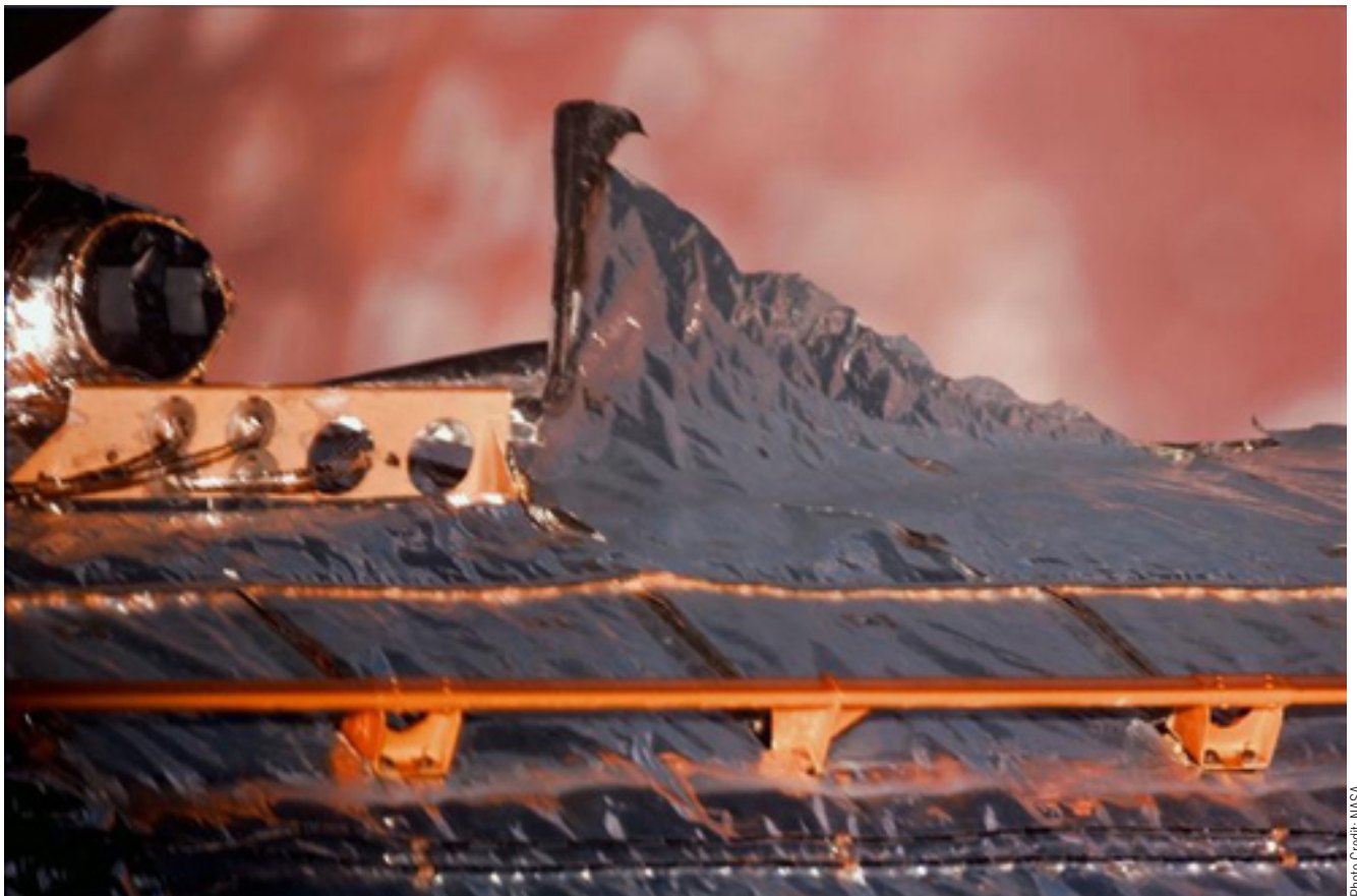
Caption: One of several tears in the outer layer of Hubble's multi-layer insulation blanket along the direct Sun-exposed side of the telescope.
