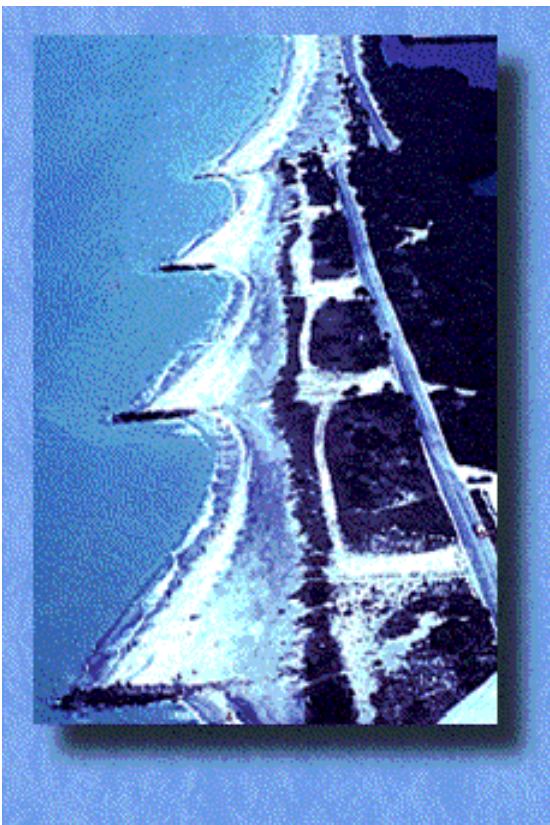
Photo 9. Shoreline stabilization structures such as groins are intended to reduce the erosion of shorelines, but in some cases may exacerbate or shift the problem to another portion of the beach.
