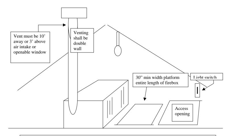
Must provide combustion air.
