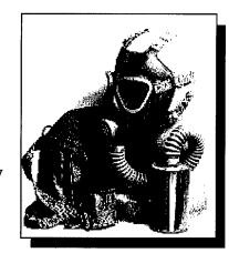
nosecup. An improved lightweight canister provided better protection. An improved outlet valve resulted in the M3A1 Mask in 1944. Over 13 million of the masks were produced during World War II. The masks were obsoleted in 1949.
