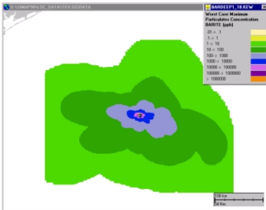
Figure 82. Peak exposure concentration (ppb) of barite as particulate in the water at each location: worst case of all simulations (Scenario 17).
