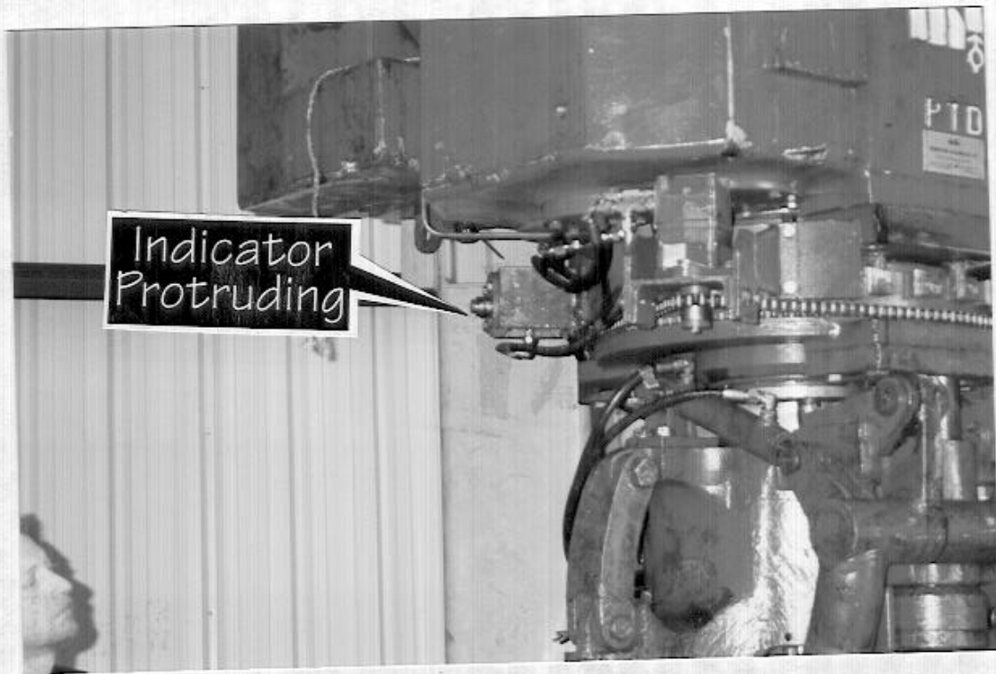
PIN DISENGAGED — INDICATOR PROTRUDING
