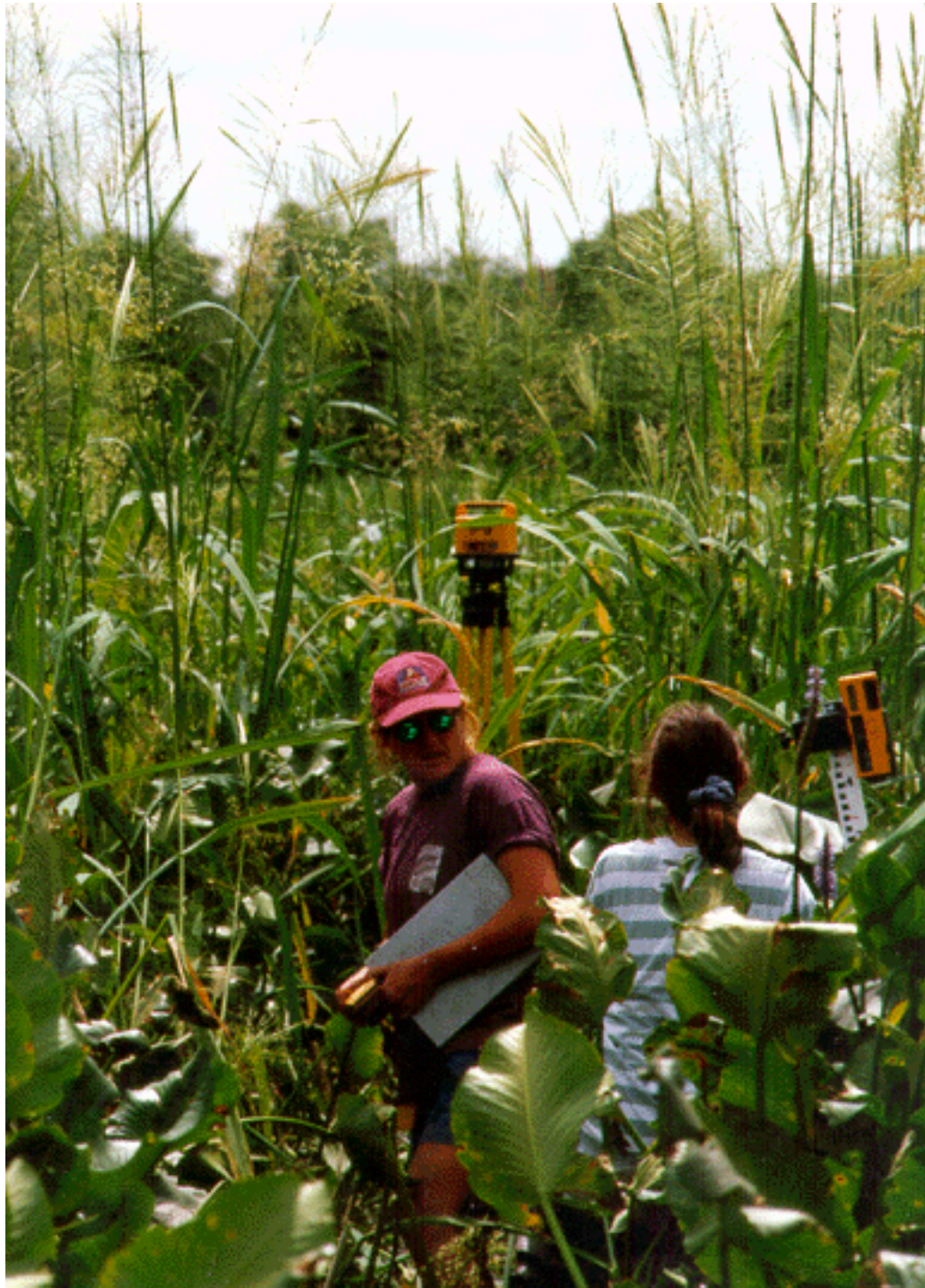
Figure 4-4. Photograph of Academy staff members surveying the elevation of the marsh at the boundary between the low marsh (foreground, dominated by broad-leaved, Nuphar ) and high marsh (background, dominated by wild rice, Zizania ).
