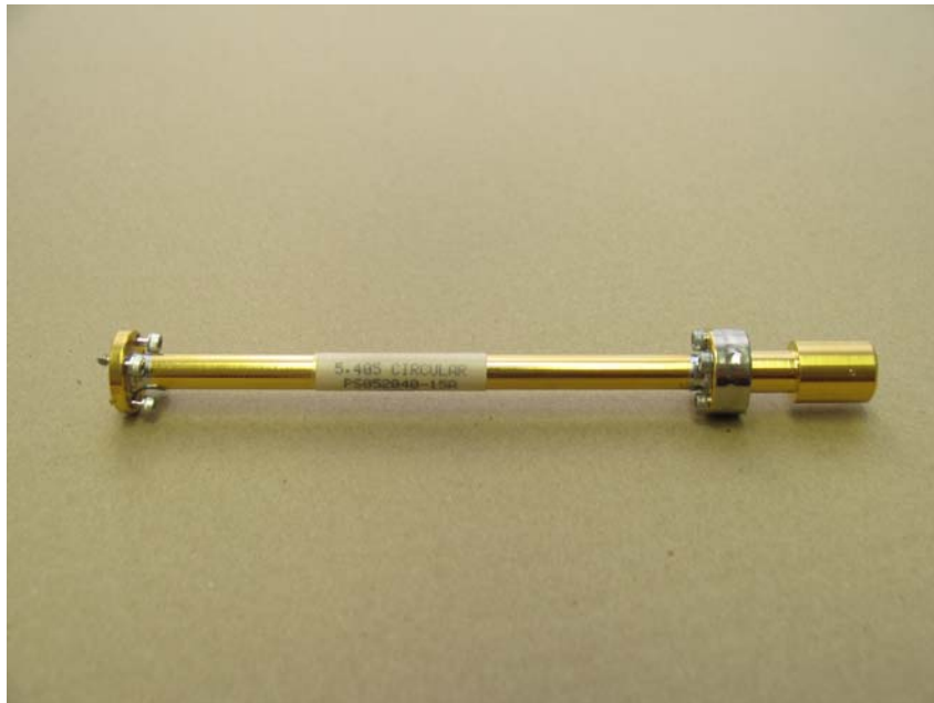
Figure 29. Cylindrical waveguide with permanently attached feed horn.
