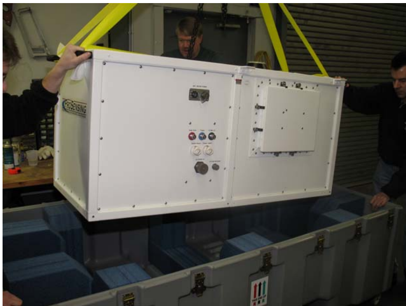
Figure 42. RF unit being lowered into shipping container by overhead hoist.
