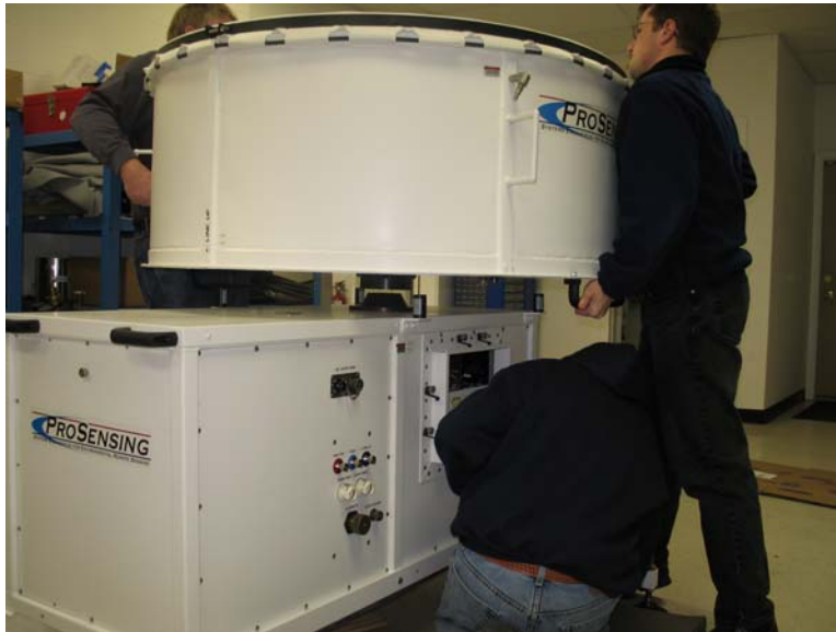
Figure 28. Lift antenna approximately 0.5” to slide waveguide into place (antenna lifted 3” in this picture).
