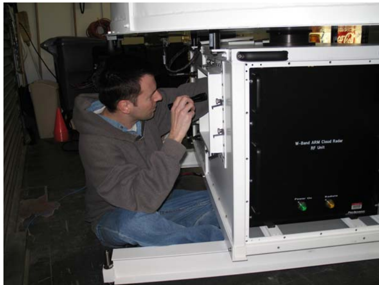
Figure 27. Access panel providing access for installing the waveguide between the RF Unit and Antenna.
