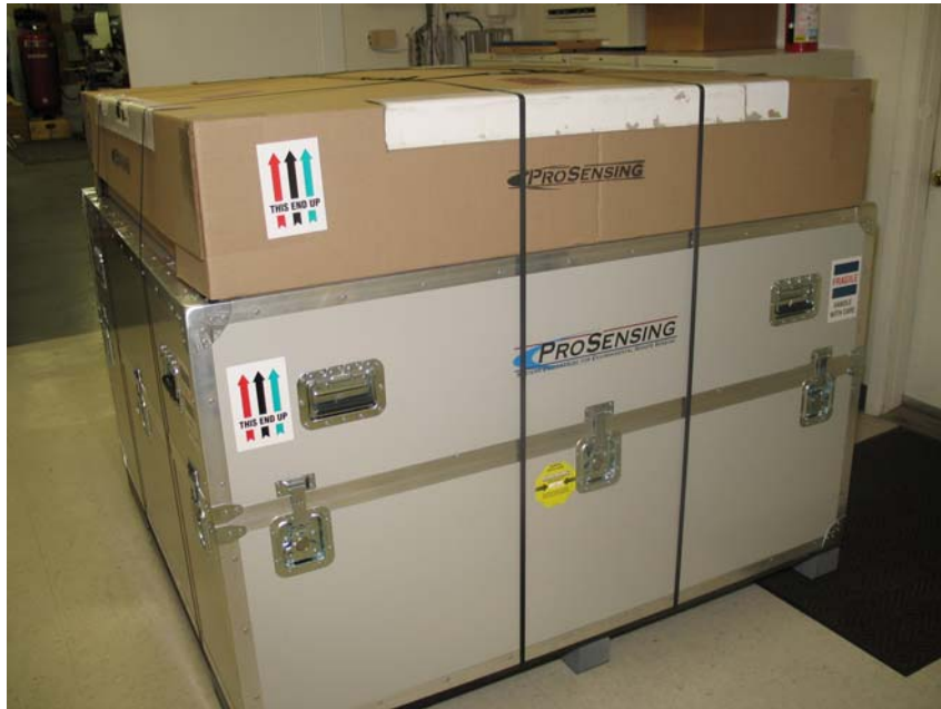
Figure 45. Environmental enclosure base and external insulation blanket are shipped in the pasteboard box secured to the top of the antenna shipping container.
