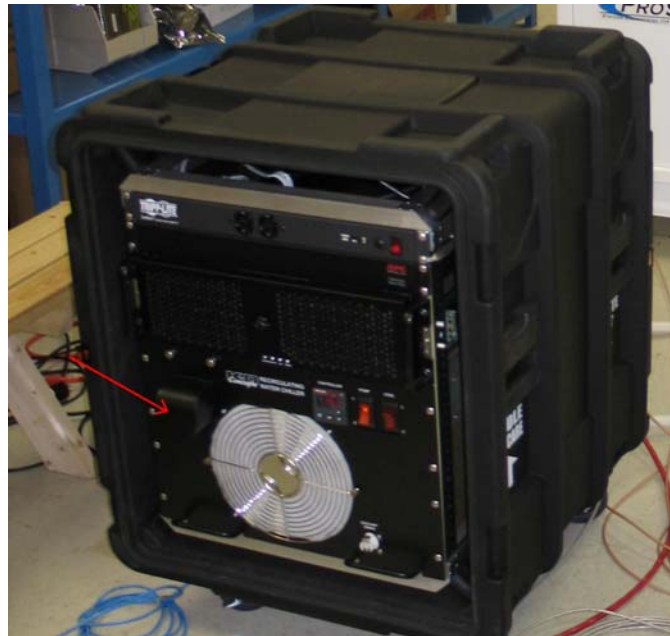
Figure 37. Chiller fill point shown with red arrow.
