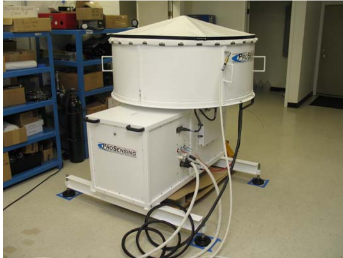
Figure 1. WACR AMF RF unit environmental enclosure and antenna housing.
