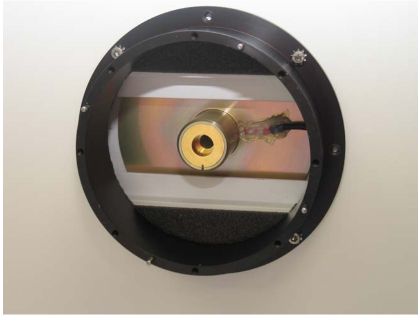
Figure 30. Feed horn inserts into cylindrical waveguide collar (gold) on base of antenna.
