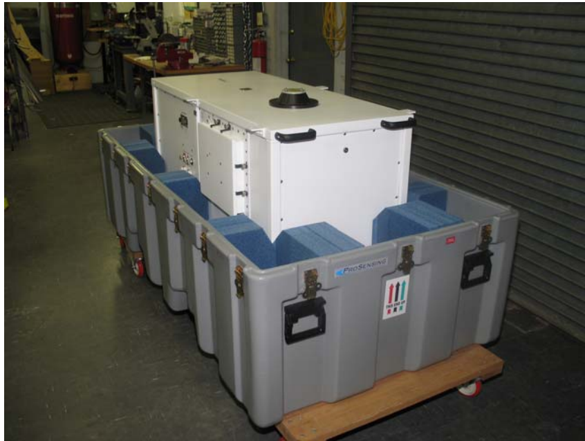
Figure 43. Environmental enclosure inside shipping container.
