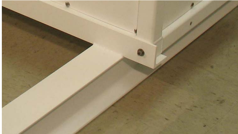
Figure 19. 1/4-20 x .75” bolt fastening Environmental Enclosure to mounting rails.
