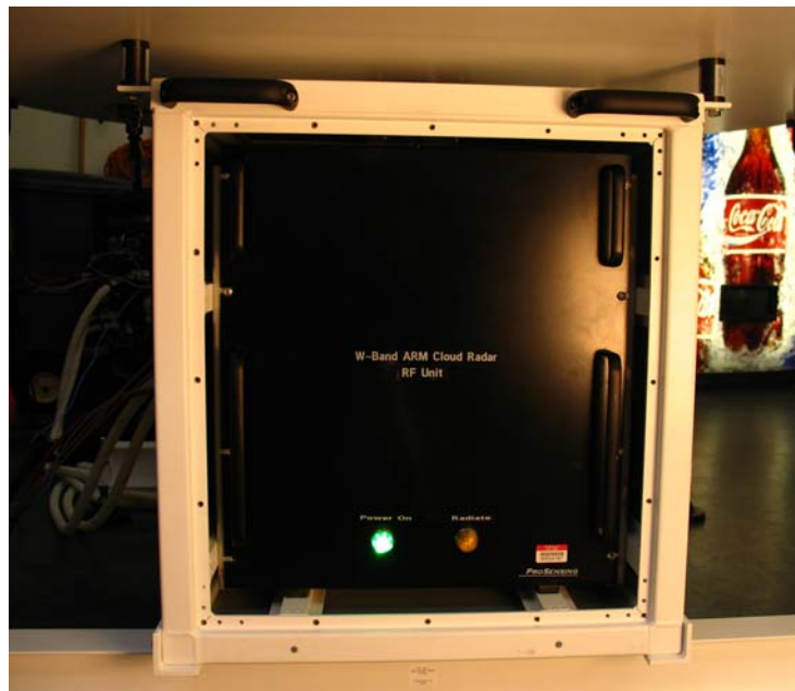
Figure 9. RF unit mounted in the Environmental Enclosure underneath the antenna.
