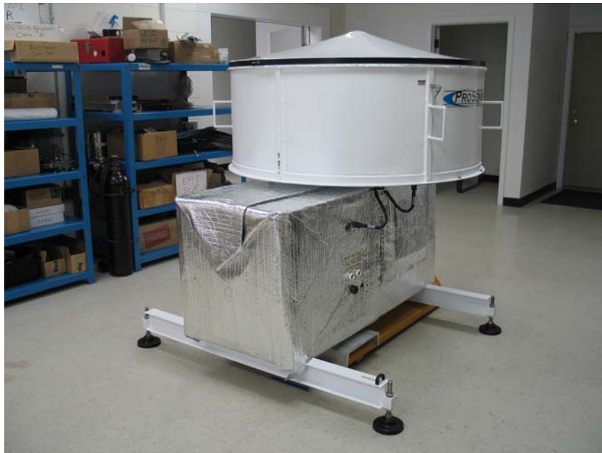
Figure 23. Temporary insulation blanket installed on RF unit environmental enclosure.
