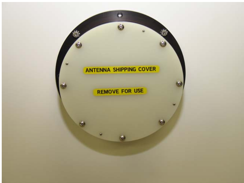
Figure 25. Protective plate covering mating rings on antenna and RF unit environmental enclosure.
