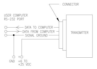
Proper connection requires identifying the correct output pins on the computer RS-232 port and on our transmitter output connector.
