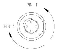
CONNECTOR PART NO.: XSE-4-BCR MATING CONNECTOR: XSE-4-CCP
