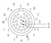
CONNECTOR PART NO.: MS3102A28-12P MATING CONNECTOR: MS3106A28-12S
