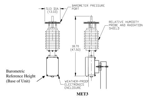
The MET3A must be installed with the barometric port assembly vertical as shown below. MET3A units that are delivered with the barometer port dismounted from the main body should be assembled in the following manner:
