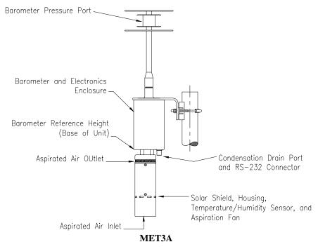
Install the unit in a location where the ports remain unobstructed. There should be at least one foot of clearance in all directions and at least four feet of clearance from the ground. The ports are designed to minimize effects caused by solar radiation and wind, and obstruction of the ports could result in erratic performance. For GPS Meteorology applications we recommend that the MET3A be installed with the barometer port at the GPS antenna height.
