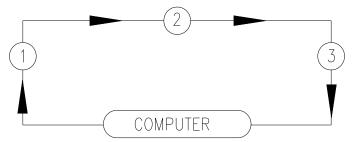
All messages move clockwise around the loop, relayed from transmitter to transmitter. Each transmitter picks off the messages addressed to it and relays responses or other messages onward.
