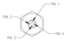
CONNECTOR PART NO.: XSG-4-BCL MATING CONNECTOR: XSG-4-CCP
