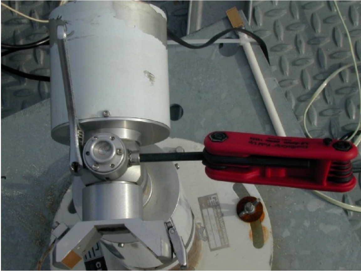
Figure 7: Adjusting zenith bolt
