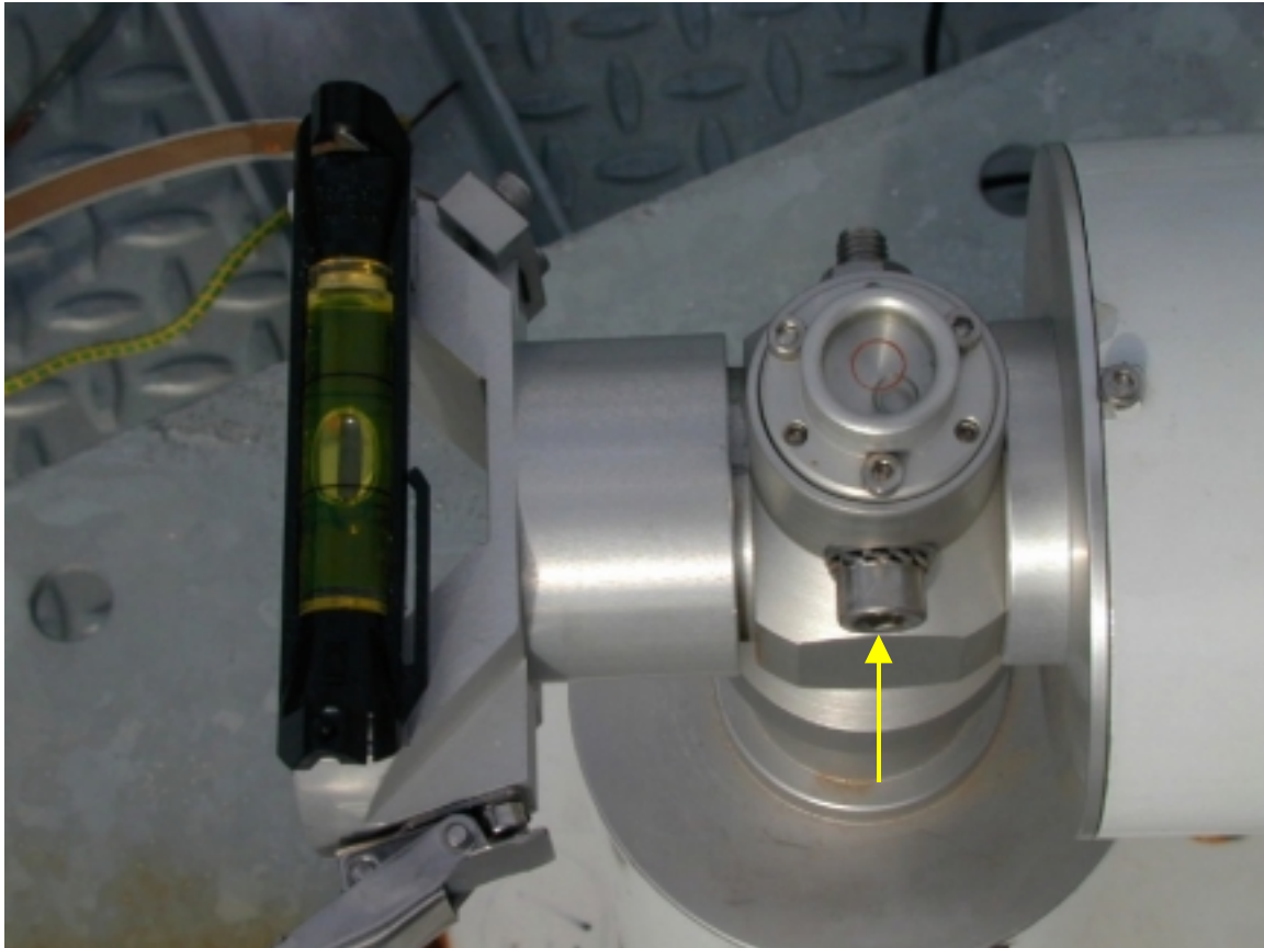
Figure 6: Zenith bolt used to adjust sensor head leveling
