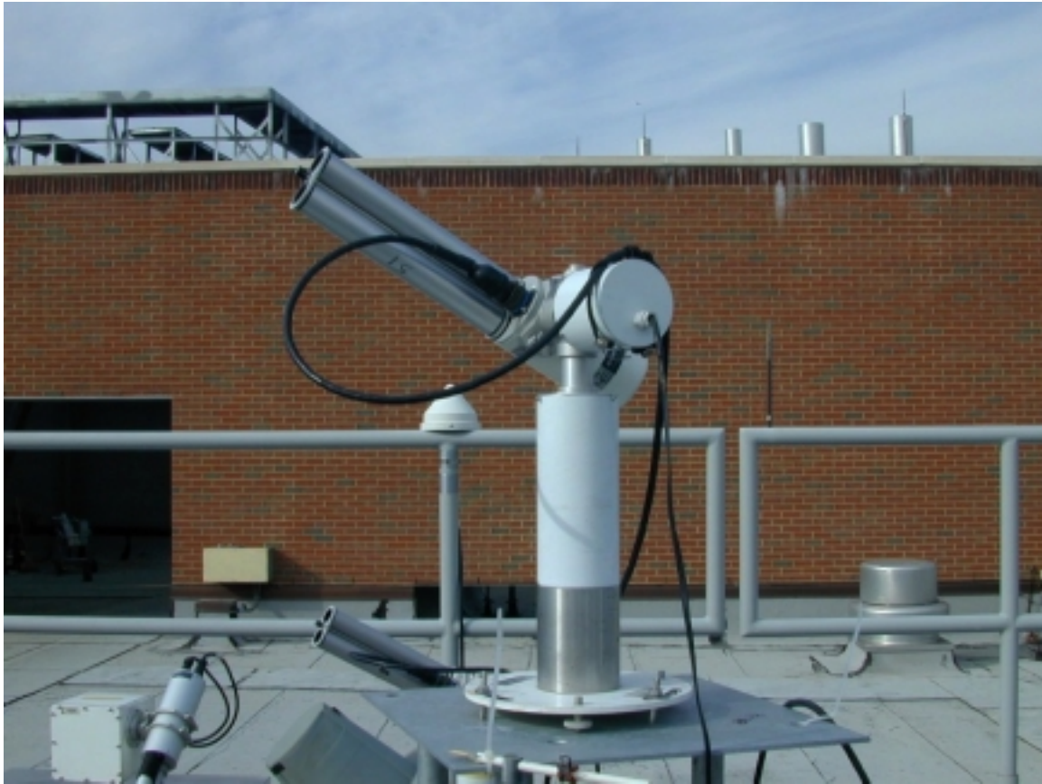
Figure 8: Cimel performing a GOSUN procedure
