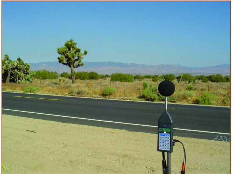
The Volpe Center developed the Traffic Noise Model (TNM) for the FHWA, which recently mandated the TNM for use for all traffic noise analysis in the United States. Above, noise measurement equipment used for “quiet pavements” research.
