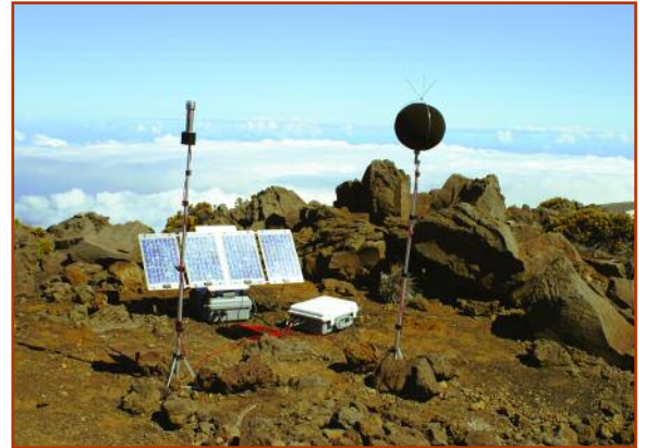
Noise measurement equipment gathers data for use by Volpe Center teams in developing acceptable and effective measures to mitigate or prevent significant adverse impacts from commercial air tours in Haleakala National Parks.
