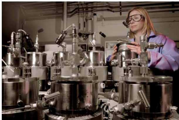
Barbara Kutchko uses a series of high-pressure vessels manufactured specifically for NETL's Geologic Sequestration Core Flow Laboratory, currently used in evaluating the potential for cement degradation to affect storage integrity for geologic storage of carbon dioxide.
