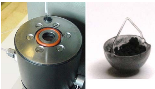
The coal-metal oxide sample in the Thermogravimetric analysis unit.
