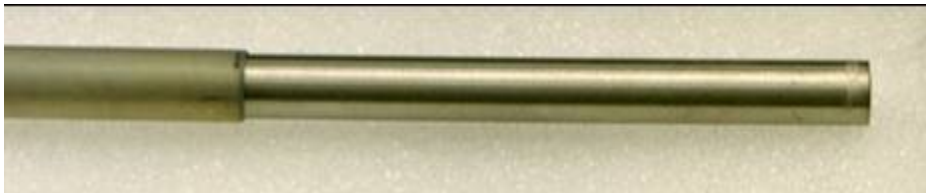
Figure 5 – Fermi-1 Blanket Rod after Sodium Removal by MEDEC Process
