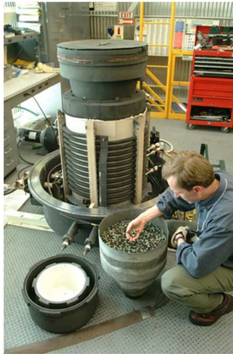
Figure 7 – Early Testing of the Prototype Metal Waste Furnace Used for Pyroprocessing
