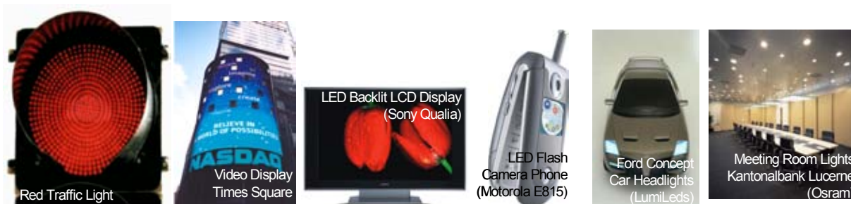
Figure A-2 Current and near-term application using high-brightness LEDs and SSL.
