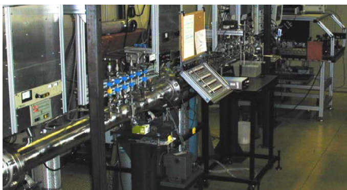
Figure 2. Shock tube at Stanford University (courtesy of Dr. D. Davidson). The silver tube running diagonally across the picture is the shock tube. Laser-based methods measure reaction rates at the far end.
