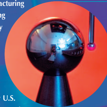
Precision sphere measurement on a coordinate measuring machine
