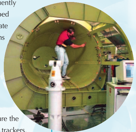
The aerospace industry uses MEL-invented and calibrated laser trackers to help them build large parts accurately
