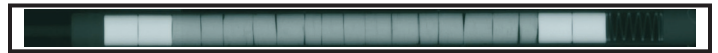
Figure 3. Neutron radiograph of 94% dUO 2 -6% RGPuO 2 -<1% NpO 2 LWR-1a MOX rodlet irradiated to 9 GWd/tU burnup.
