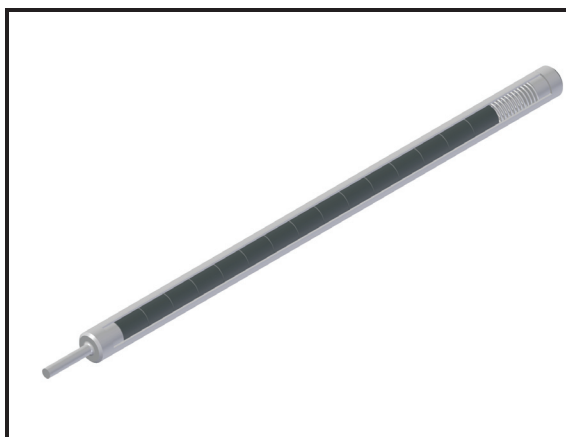
Figure 4. 3-D representation of LWR-2 fuel irradiation test pin.
