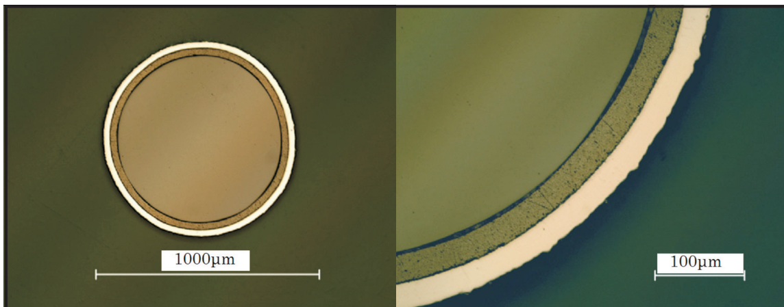
Figure 3. Optical micrographs of the developmental IPyC and ZrC coatings on surrogate zirconia kernel.
