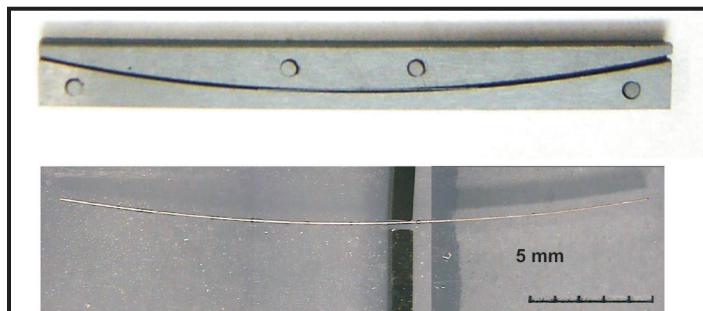
Figure 1. Bend stress relaxation holder assembly for irradiation creep study of refractory ceramics (upper), and ZrC sample after creep deformation to 3.7 dpa at 640°C.
