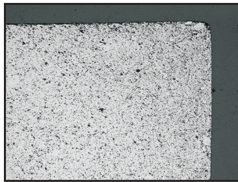
Figure 1. Low-fertile optical micrograph of axial pellet section.
