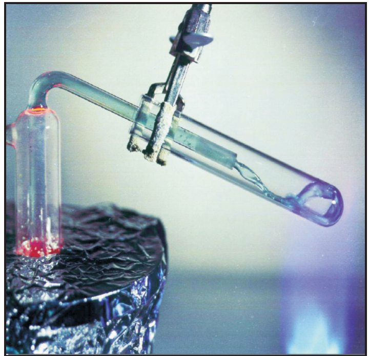
Figure 1. Liquid salts are being investigated as possible heat transfer media.
