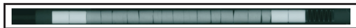
Figure 4. Neutron radiograph of 94% dUO 2 – 6% RGPuO 2 – <1% NpO 2 sample PROF-3 irradiated to ~9 GWd/tU burnup.
