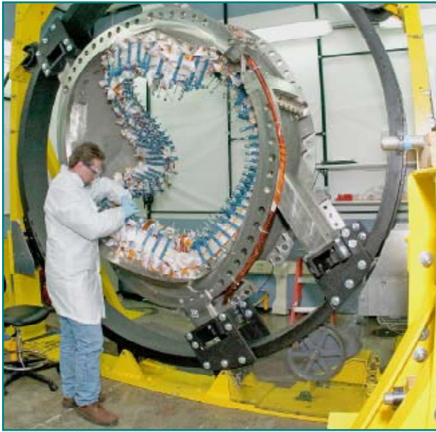
Figure 5. Winding of an NCSX modular field coil.
