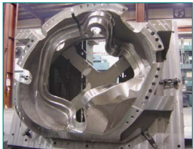
Figure 4. Modular field coil winding form.
