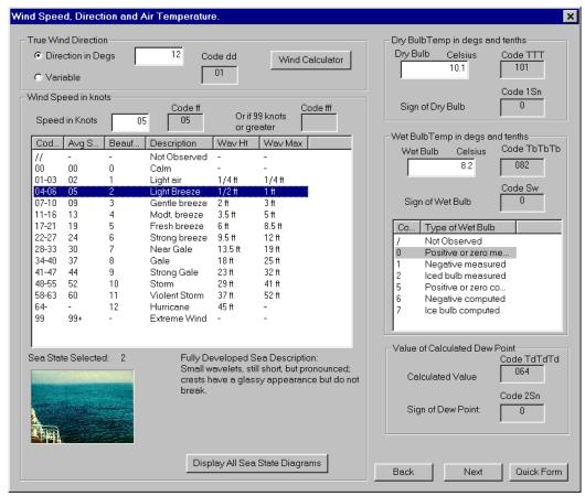
Figure 7. Wind speed, direction and air temperature screen
