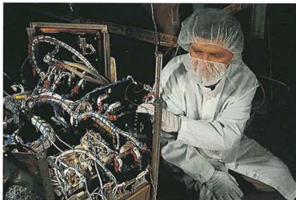
Eli Abronovich, Principal Mechanical Engineer at CTA Space Systems, connects a momentum wheel to a commercial space satellite. Several reaction/momentum wheels can be used to provide full three-axis attitude control and stability.
