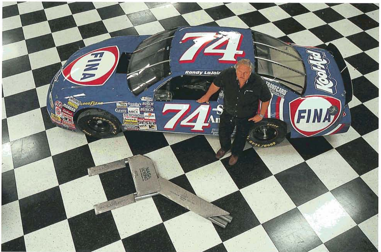
Butch Stevens of BSR Products, Inc., lays out a custom exhaust thermal protection system in front of the Motorsports Busch Grand National race car. BSR created blanket insulation kits based on NASA Space Shuttle Thermal Protection System materials and had the first products bear a seal from the U.S. Space Foundation indicating their space origin.
