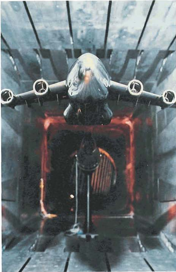
An airplane model is tested in Langley's National Transonic Facility, one of Langley's many wind tunnels.
