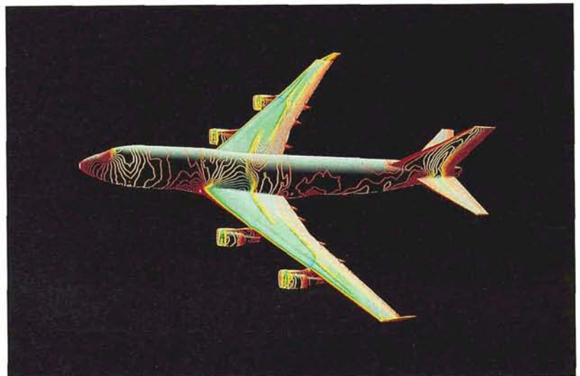
Langley was a recipient of NASA's 1996 Software of the Year award for the Tetrahedral Unstructured Software System (TetrUSS), an aerodynamic analysis and design system used here on the Boeing 747 to study aerodynamics and other problems.
