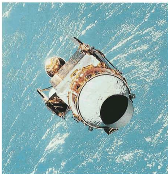
NASA's Advanced Communications Technology Satellite (ACTS) is the technology leader of satellite communications, using futuristic dynamic hopping beams and advanced on-board switching and processing.
