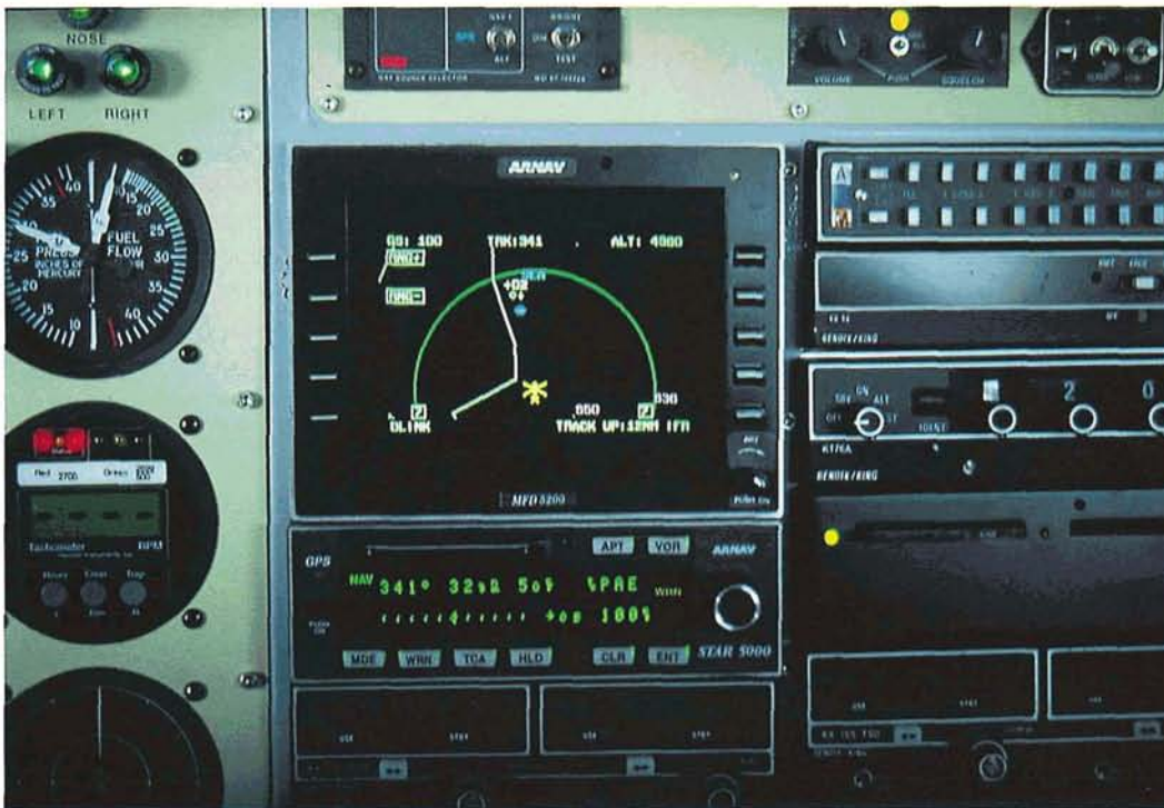
ARNAV Systems, Inc. was one of the private companies involved in an Olympic demonstration of new air traffic control technologies. Their system was used to provide automatic dependent surveillance-broadcast capability for aircraft operating within FAA temporary flight restricted areas.
