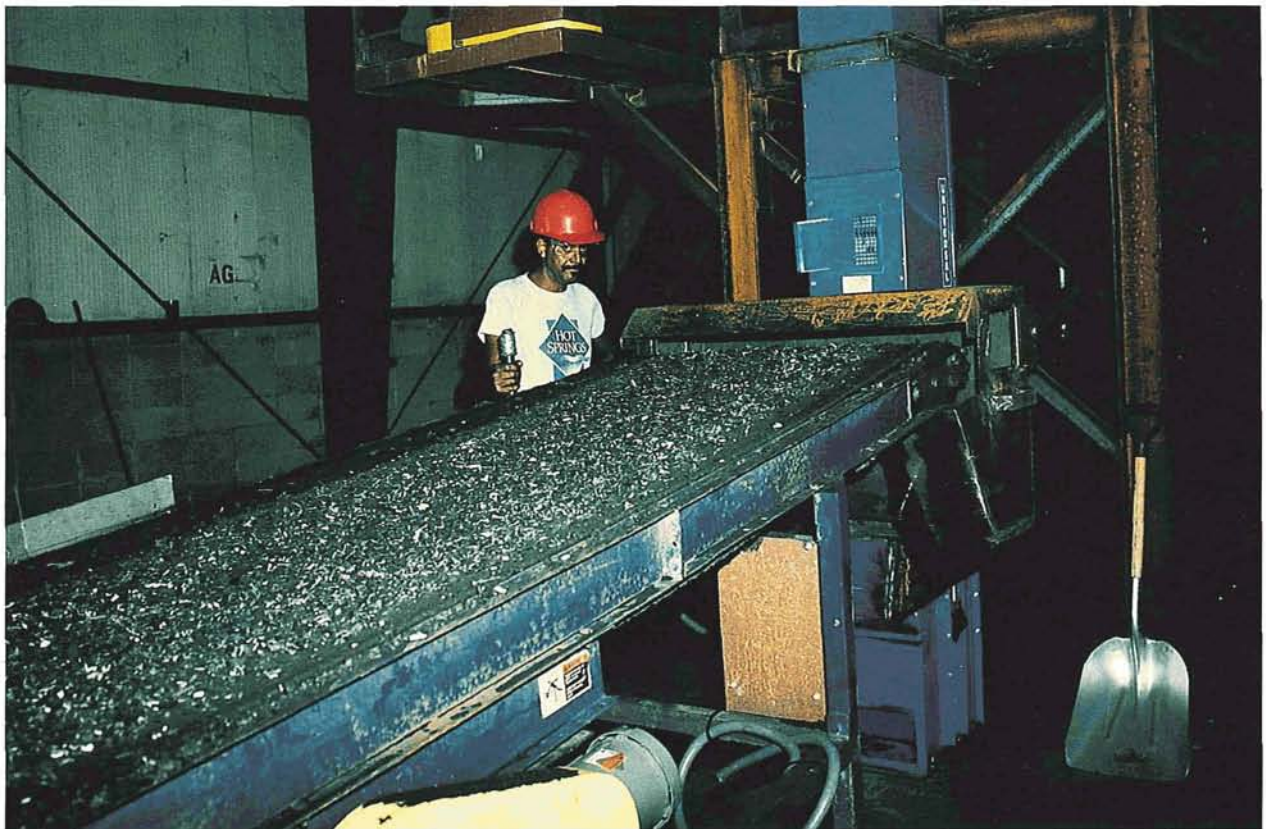
Recycled tire “crumbs” help reduce tire disposal problems and are used in asphalt roadbeds and other items. NASA experts on cryogenic equipment made the recycling idea more cost effective.
