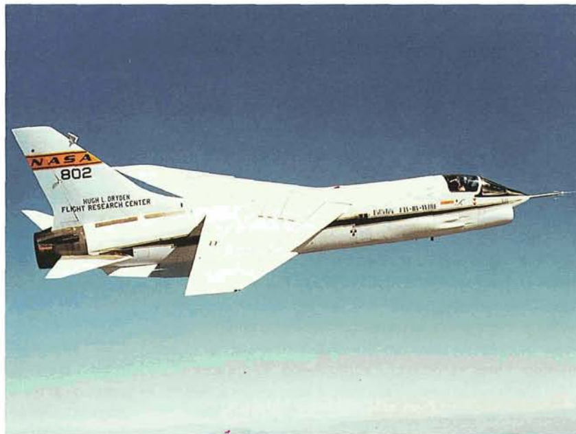
NASA F-8 Digital Fly-By-Wire research aircraft is on one of its pioneering flights in the 1970s. Dryden-led research developed electronic fly-by-wire flight control systems used in many aircraft today, including the Space Shuttle orbiters.
