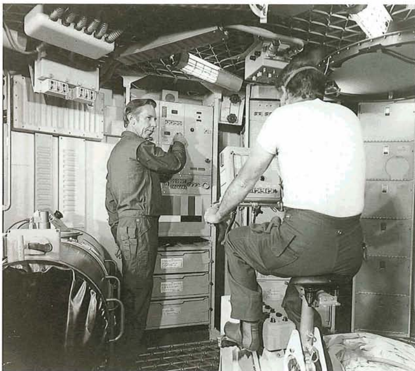
In 1973, an engineer set controls as a second engineer uses Ergometer in the full-scale mockup of the Orbital Workshop at Marshall Space Flight Center. The workshop is the largest component of Skylab.
