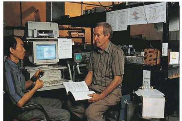
Graduate student Han-Sun Choi (left) and Dr. Henry Taylor of Texas A&M University test fiber optic temperature sensors. FFPI Industries tests each of its sensors on an engine with a computer calibration system before shipping.
