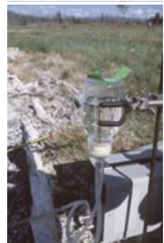
Figure 4. Field-portable, bubble-stripping apparatus for measurement of H_2 in geothermal waters. An intake tube is wrapped in insulation to keep the water hot. A peristaltic pump pumps water through a glass jar (right) with a 20-ml atmospheric air bubble inside. After an amount of pump time at a given rate of flow, the bubble is withdrawn for analysis.
