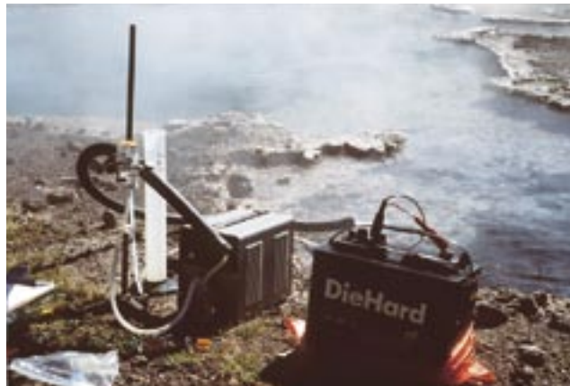
Figure 4. Field-portable, bubble-stripping apparatus for measurement of H_2 in geothermal waters. An intake tube is wrapped in insulation to keep the water hot. A peristaltic pump pumps water through a glass jar (right) with a 20-ml atmospheric air bubble inside. After an amount of pump time at a given rate of flow, the bubble is withdrawn for analysis.
