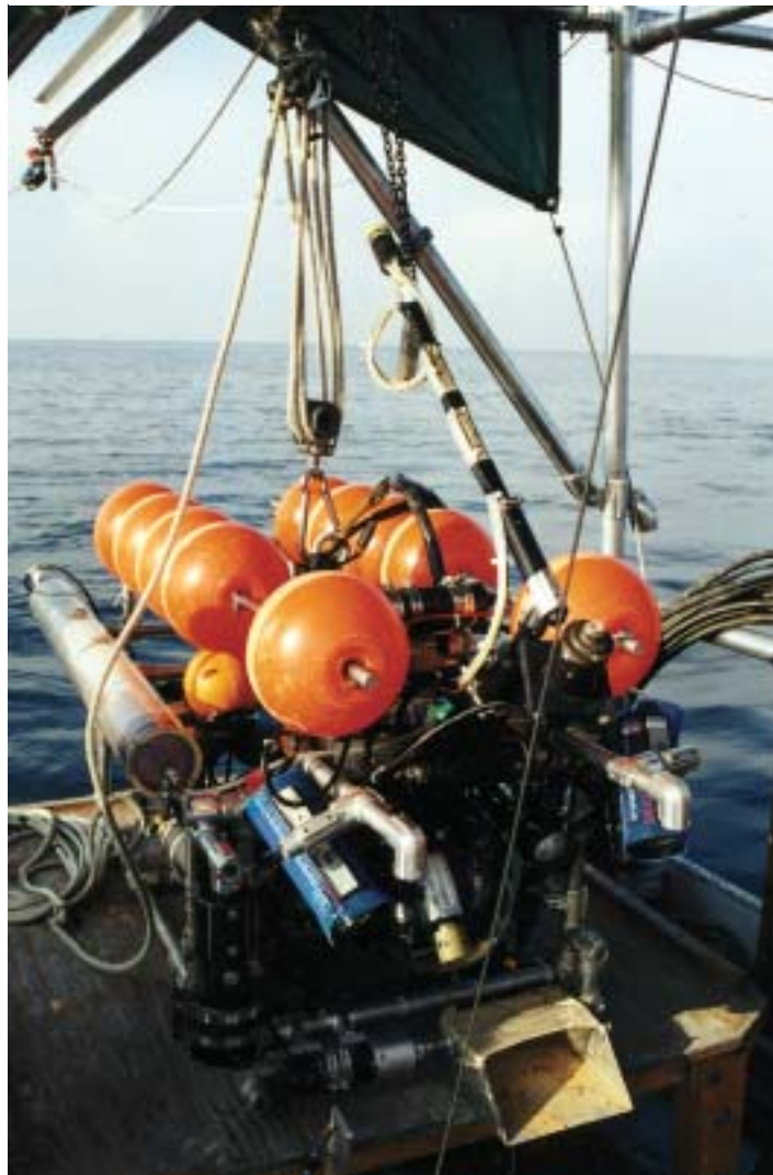
Remotely-operated vehicle (ROV). The large orange balls are flotation units. Water samples are drawn through the large tube mounted on the left. A thermometer/camera is visible in the mid-foreground, directly above the basket used for scooping up sediment samples from the lake floor.
