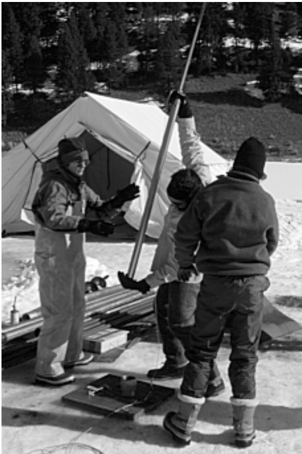
Winter is the ideal time of year to conduct this coring operation because the lake's frozen surface allows researchers to core into the deepest parts of the lake without using a boat. NPS photo.
