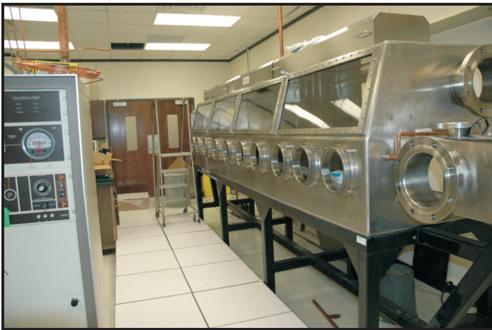
Figure 1. Glovebox installed at TAMU for powder metallurgy of U alloys.
