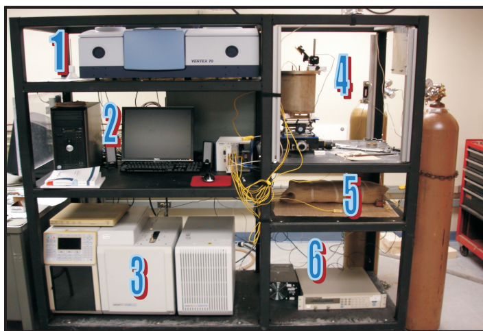
Figure 2. Status of the construction of the emissivity measurement system: (1) FTIR spectrometer; (2) data acquisition system; (3) mass spectrometer/gas chromatograph; (4) location of furnace with isothermal silicon carbide sample holding block; (5) gas preheating coil; (6) voltage sources for gas preheater and valves.
