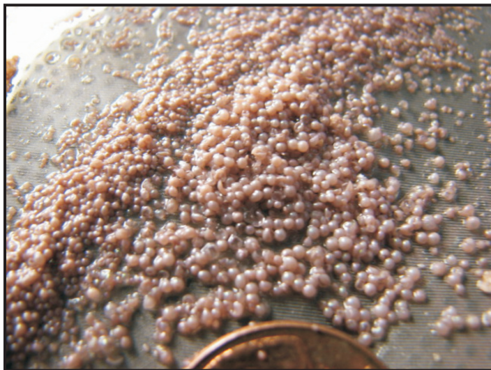
Figure 1. Cerium oxide microspheres fabricated via internal gelation.
