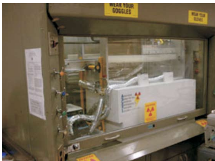
Figure 4. The ASCEFI system inside a radiological fume hood.
