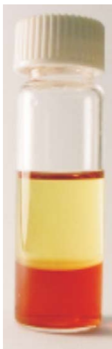
Figure 4. Distribution of uranium between aqueous phase (orange-red complex of uranyl-hydraxamate, bottom phase) and organic phase (uranium nitrate in 30 percent TBP in n-dodecane, upper phase).
