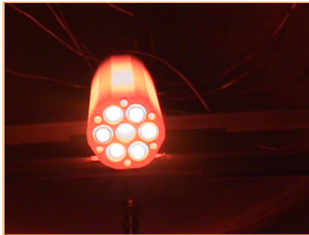
Figure 16. Heat pipe fission reactor research for space applications is ongoing at Los Alamos National Laboratory
